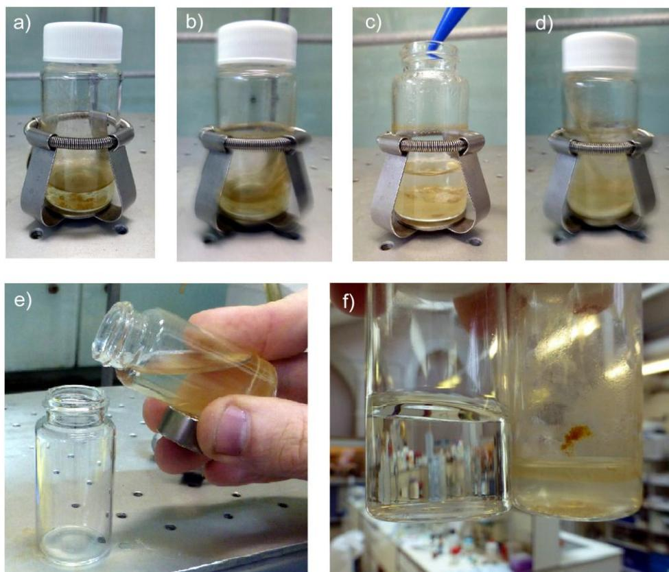
a) Catalyst  $\text{Fe}_3\text{O}_4/\text{Si}[\text{CuI}(\mathbf{5})]$  in water with azide and alkyne; b) reaction shaken overnight; c) ethyl acetate added to dissolve triazole formed; d) vial shaken for a few minutes; e) organic layer decanted using hand-held magnet; f) organic and aqueous components.
