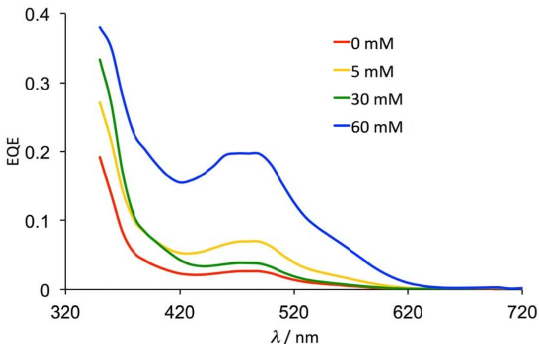
Fig. S1. EQE (IPCE) spectra for DSCs detailed at the top of Table 2 (main text) containing  $[\text{Cu}(\mathbf{3})(\mathbf{4})]^+$  dye and  $[\text{Co}(\text{bpy})_3]^{2+}/[\text{Co}(\text{bpy})_3]^{3+}$  electrolyte. In three cells (green, yellow and blue lines), the  $\text{TiO}_2$  was post-treated with aqueous  $\text{TiCl}_4$  using solutions of 5, 30 and 60  $\text{mmol dm}^{-3}$ . The red line corresponds to no post-treatment.
