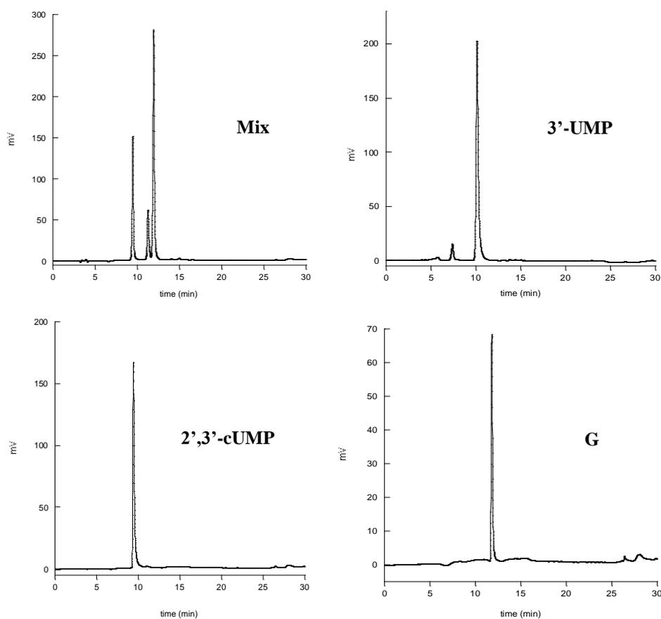
**Figure S5:** Verification of cleavage products after complete cleavage (Mix, 6-fold higher conc. (0.3 U/ml) of RNase A after 30 s) by comparison to commercial guanosine (G), uridine 3'-phosphate (3'-UMP) and uridine 2',3'-cyclic phosphate (2',3'-cUMP).
