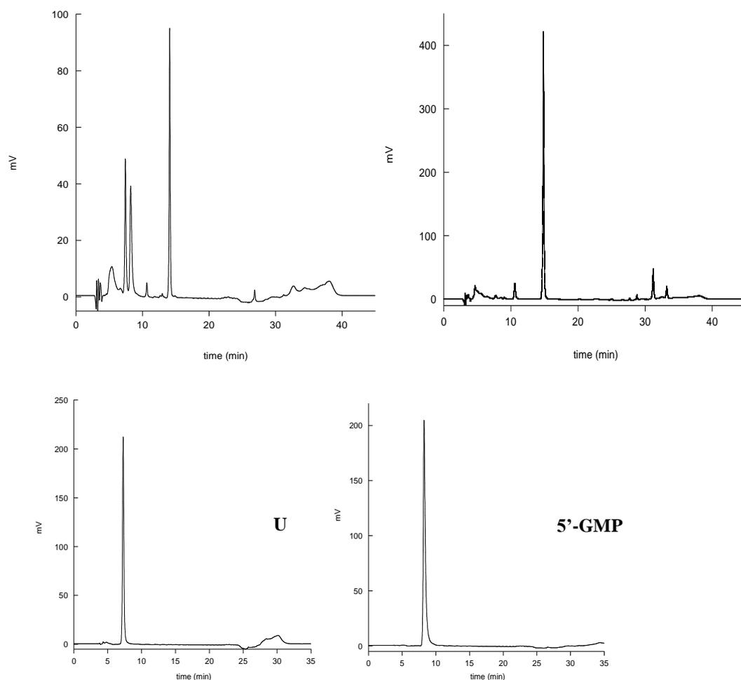
**Figure S2:** Upper left panel: Treatment of UpG with PDE I after 5 min of incubation; Upper right panel: Treatment of UCH<sub>2</sub>pG with PDE I after 2 days incubation. The RP-chromatogram shows that there is no degradation of the modified dimer when incubated with the enzyme. Lower left panel: HPLC-analysis of uridine (U). Lower right panel: HPLC-analysis of guanosine 5'-phosphate (5'-GMP)
