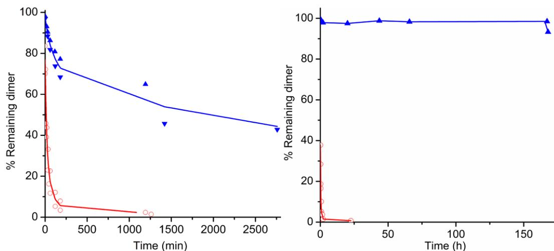
**Figure S1.** Graphs showing % remaining dinucleotide (UCH<sub>2</sub>pG in blue and UpG in red) at different times, when subjected to Spleen exonuclease, PDE II (left panel) or RNase A (right panel) at 37 °C. Quantification of dinucleotide and product was done by integration of the RP-HPLC analysis of the mixtures.
