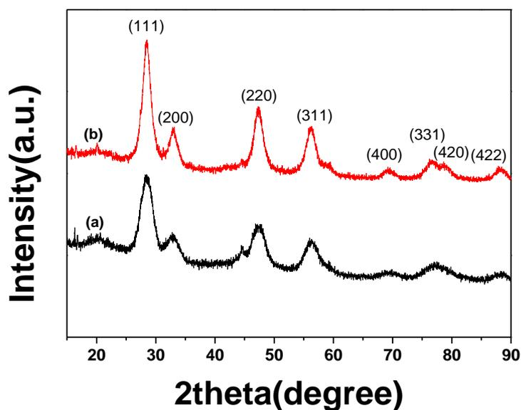
Fig. S1 XRD patterns of the as-prepared (a) ceria nanoparticles and (b) ceria nanocubes.
