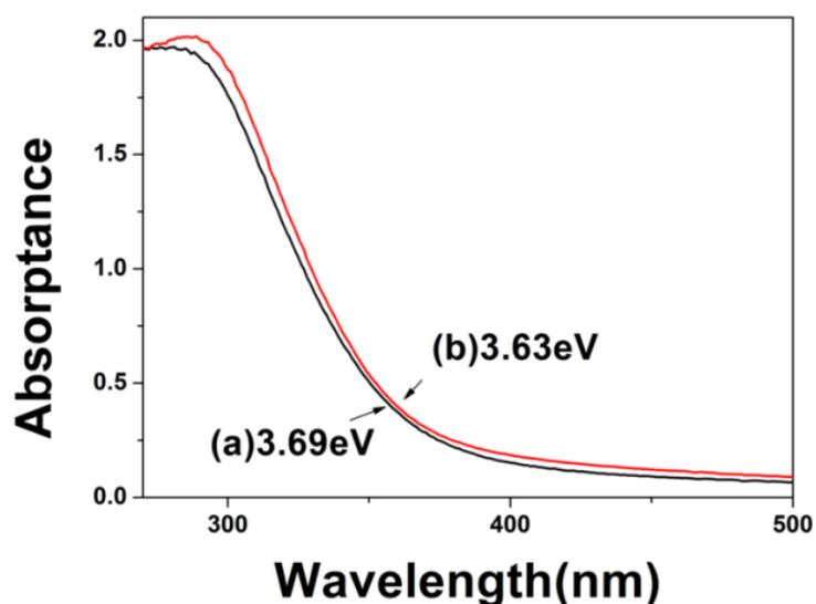
Fig. S2 The adsorption spectra for as-prepared (a) ceria NPs and (b) ceria NCs.
