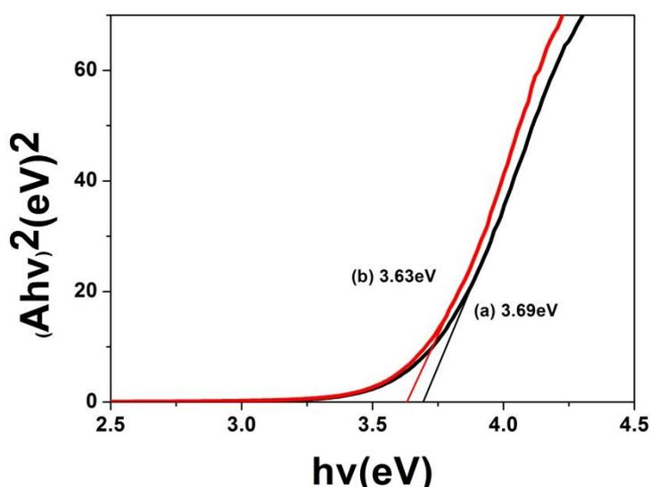
Fig. S3 Plot of  $(\alpha h\nu)^2$  versus  $h\nu$  for as prepared (a) ceria nanoparticles and (b) ceria nanocubes.
