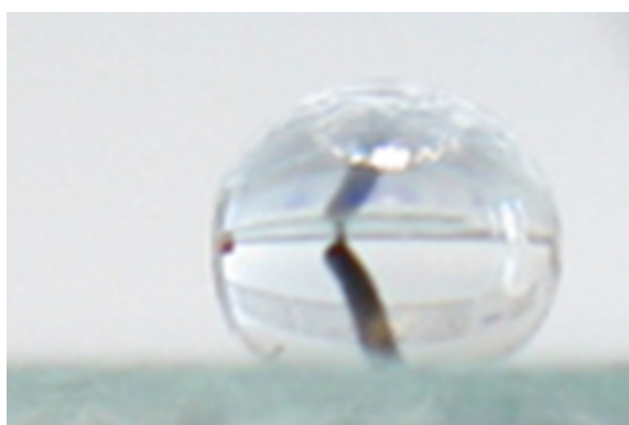
Figure S4. Water droplet (15 µL) on the surface of the SiO 2 -F coated glass slide showing the superhydrophobicity.
