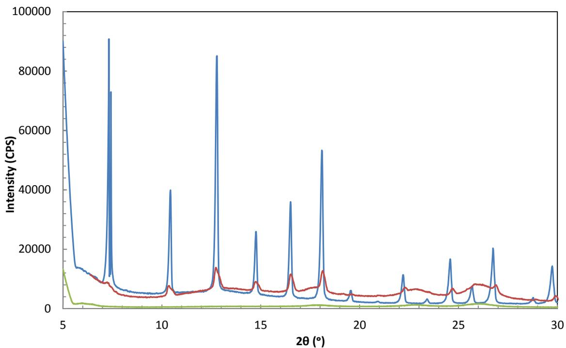
Fig. S2 X-ray diffractogram of ZIF-8 powder (blue), ZIF-8 membrane (red) and mixed-matrix support (green).
