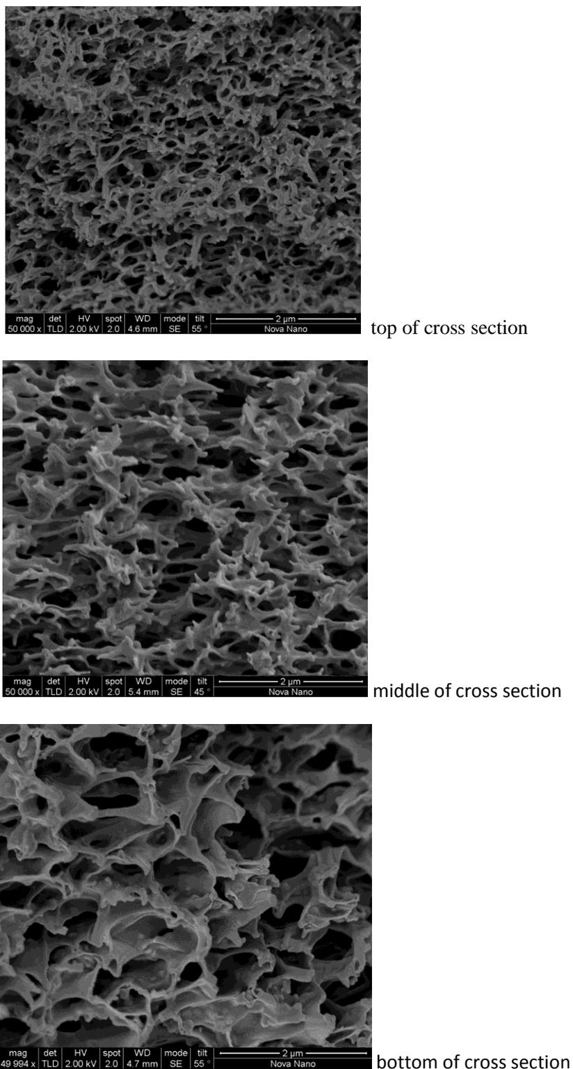
Fig. S1. SEM images of cross section of PEI/ZnO mixed matrix membrane with 40 wt % ZnO loading
