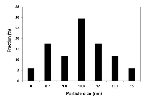
Particle size histogram of the tC-dots. The size was measured from TEM images. The particle size distribution of the tC-dots was analyzed using 95 particles from 10 TEM images.
