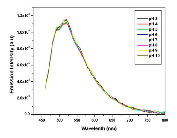
Effect of pH value on the tC-dots fluorescence. Maximum emission was taken from the excitation at 420 nm between pH 3 and pH10.
