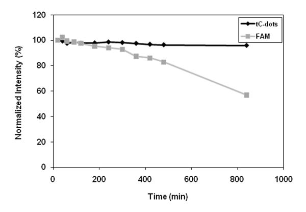
Optical stability of the tC-dots. One of the traditional dye, FAM, was used as a control. The fluorescence intensities of both the tC-dots and the FAM were acquired at the excitation wavelength of 420 nm for 14 hrs.
