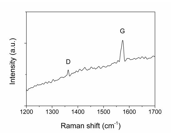
Raman spectra of tC-dots at 532 nm excitation wavelength. Raman spectra of the tC-dots showed both the G band at 1590 cm<sup>-1</sup> and the D band at 1320 cm<sup>-1</sup> which indicate sp2 and sp3 carbon, respectively.
