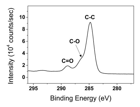
High-resolution XPS C1s spectrum of the tC-dots. The C-C, C-O and C=O carbon peak were clearly absorbed at 284.7, 286.4 and 288.8 eV, respectively.
