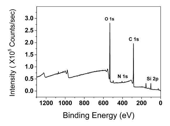
XPS spectra of the tC-dots. The spectra confirmed the presence of elements as Carbon (C), Oxygen (O), Nitrogen (N) and Silicon (Si) with the composition of 31, 58, 2 and 9 atom %, respectively.
