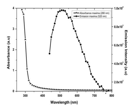
UV/Vis absorbance and emission spectra of the tC-dots. The maximum absorbance of the tC-dots was 280 nm and the maximum emission was 520 nm.
