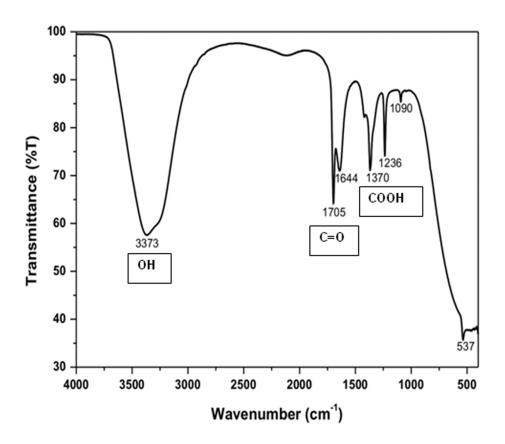
FTIR spectrum of the tC-dots. The peak of the spectrum at 3373, 1705, 1644, 1370, 1236, 1090 and 537 cm<sup>-1</sup> indicated OH, C=O, H<sub>2</sub>O, COOH, aryl-O, C-O and iodine, respectively.
