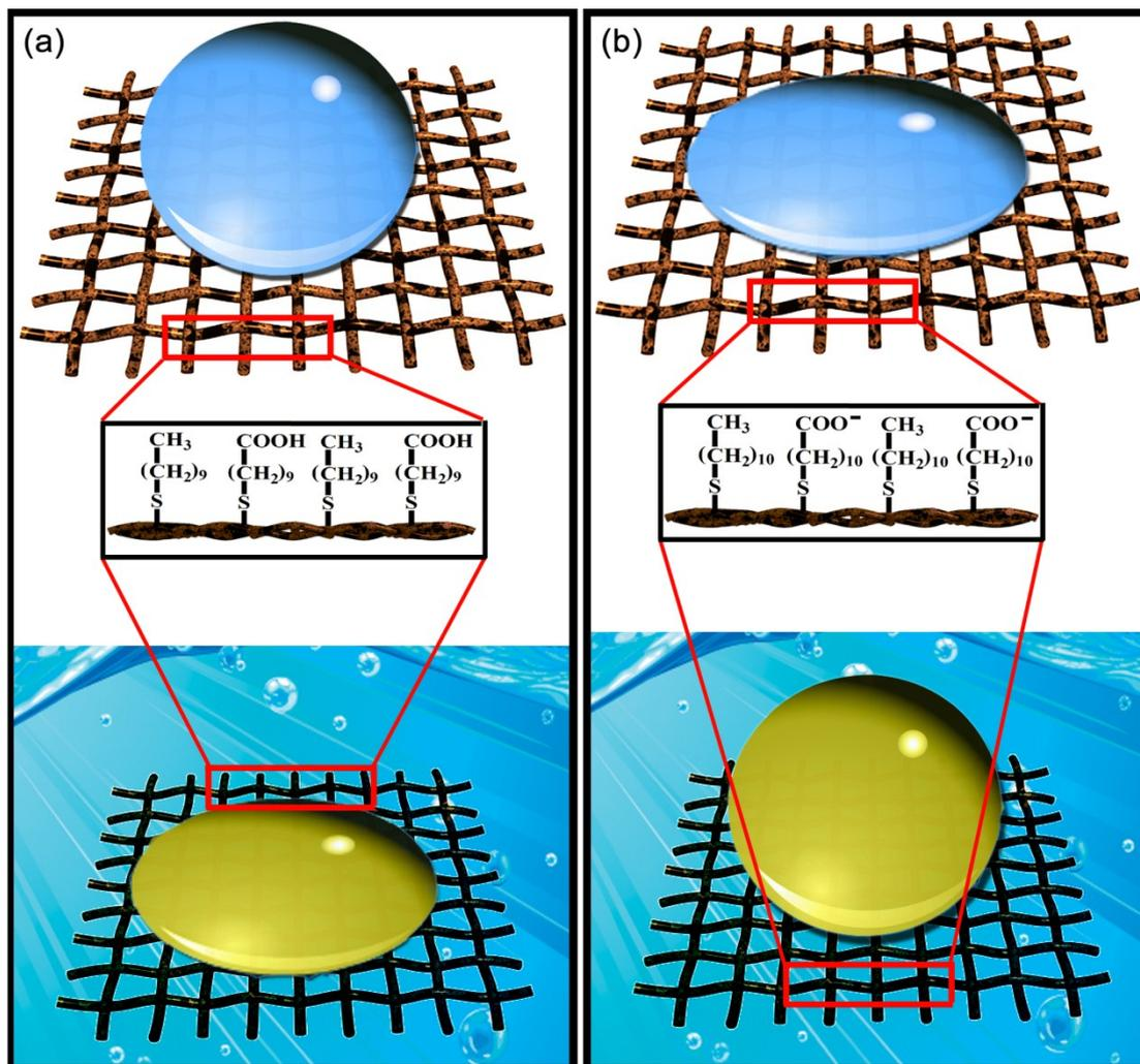
**Fig. S1** Schematic illustration of the shapes of the water droplets on the as-prepared copper mesh both in the air and underwater environment. (a) As-prepared copper mesh shows superhydrophobic property in the air to acidic and neutral water droplets however shows superoleophilic property underwater. (b) As-prepared copper mesh shows superhydrophilic property in the air to basic water droplets however shows superoleophobic property under base solution.
