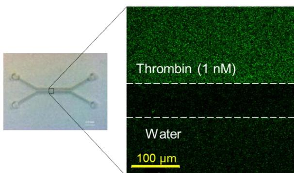
**Fig. S4** Fluorescence image of the dual-channel aptasensor prepared with a T0/T20 probe after injecting thrombin solution (~1 nM, 37 ng/mL) and water into the top and bottom channels obtained in an area including two whole microchannels.
