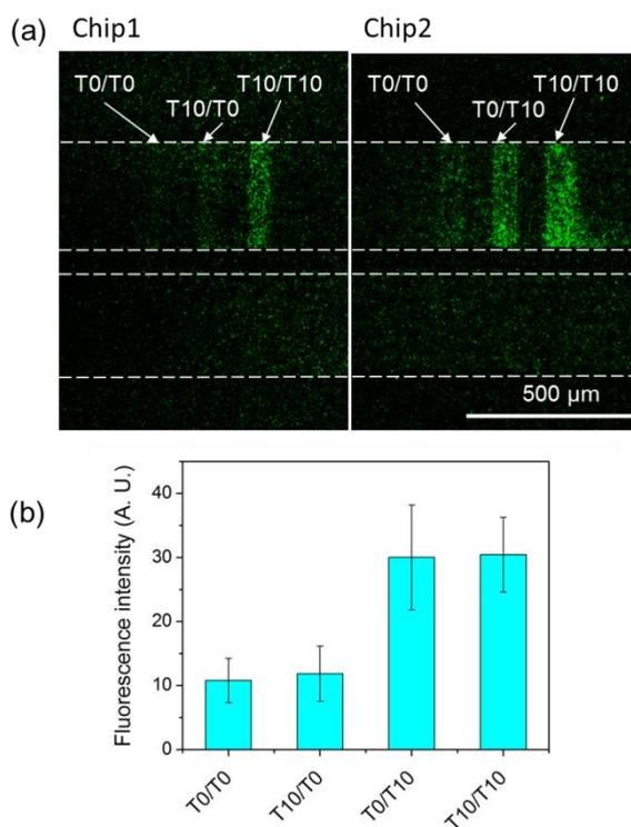
**Fig. S1** (a) Fluorescence image of 2×3 multichannel linear-array aptasensors patterned with T0/T0, T10/T0 and T10/T10 (chip 1, left) and T0/T0, T0/T10 and T10/T10 (chip 2, right). Thrombin solution (100 μg/mL) and water were injected into the top and bottom microchannels. (b) Comparison of the average fluorescence intensities of the patterned area in the top microchannel. The error bars corresponds to the standard deviations. The data for chips 1 and 2 were merged.
