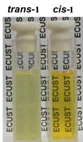
Fig. S11 Solubility variation of compound 1 in liposome contained HEPES buffer solution before (left) and after the irradiation of 365 nm light (right) (8 mW/cm 2 , 10 min).
