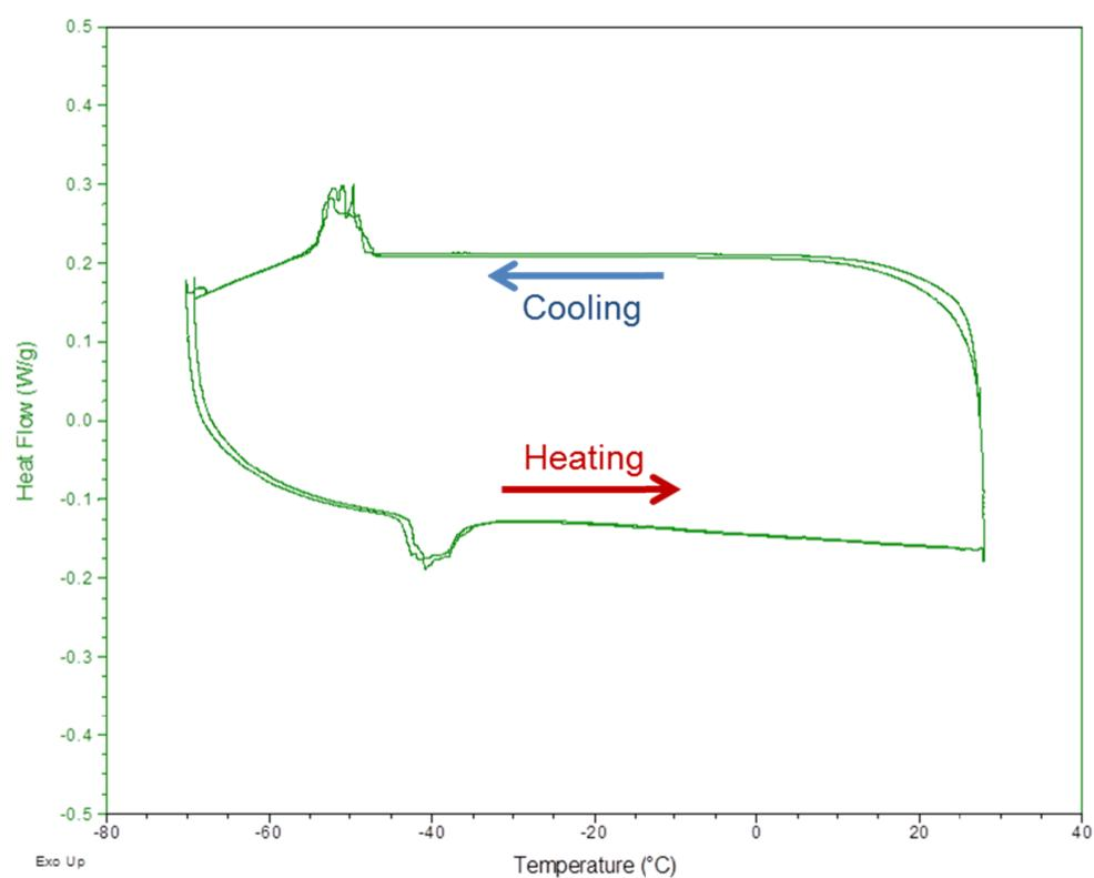
**Figure S5:** DSC analysis for **1**. Two successive cooling/heating cycles are shown.
