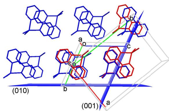
**Figure S2:** Crystal structure of 1HT (red) and 1LT (blue) viewed along the *c* and *a* axis respectively. The monoclinic and triclinic unit cells, as well as the (0 0 1) and (0 1 0) planes relative to the triclinic form, are shown.
