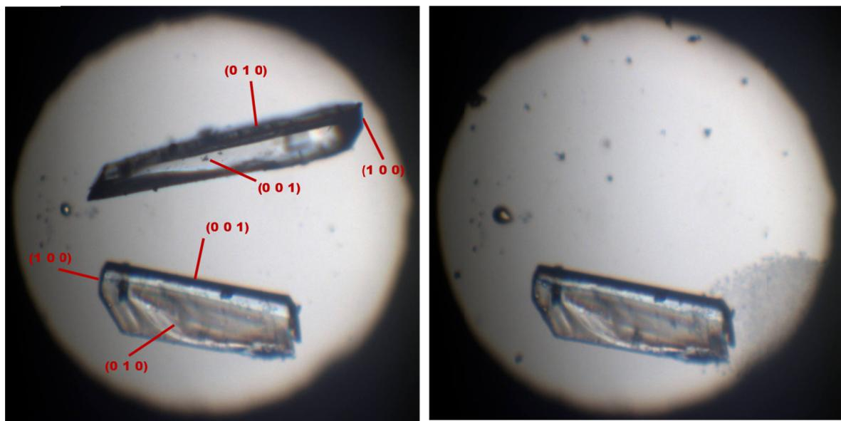
**Figure S1:** Crystals of 1 as seen on an optical microscope during the variable temperature experiment. The principal crystal faces are indicated,
