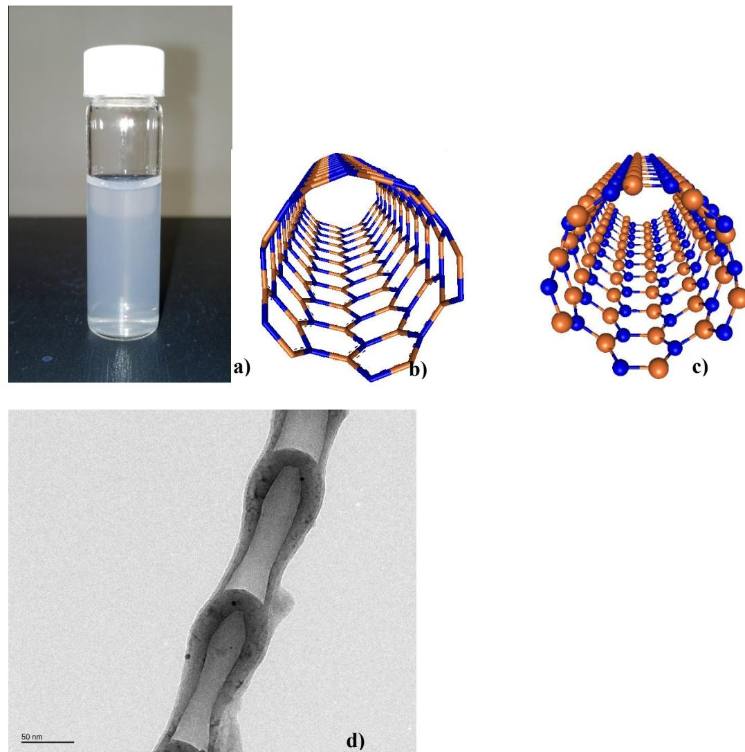
**Fig. S1** a) The photo image of BNNT suspension in water; b, c) optimized geometries for BNNT, blue and yellow atoms represent N and B atoms, as a structural analogue to carbon nanotubes (CNTs), BNNTs have boron and nitrogen atoms distributed equally in hexagonal rings; d) TEM image of BNNTs, their resolutions were 50 nm and 20 nm respectively.
