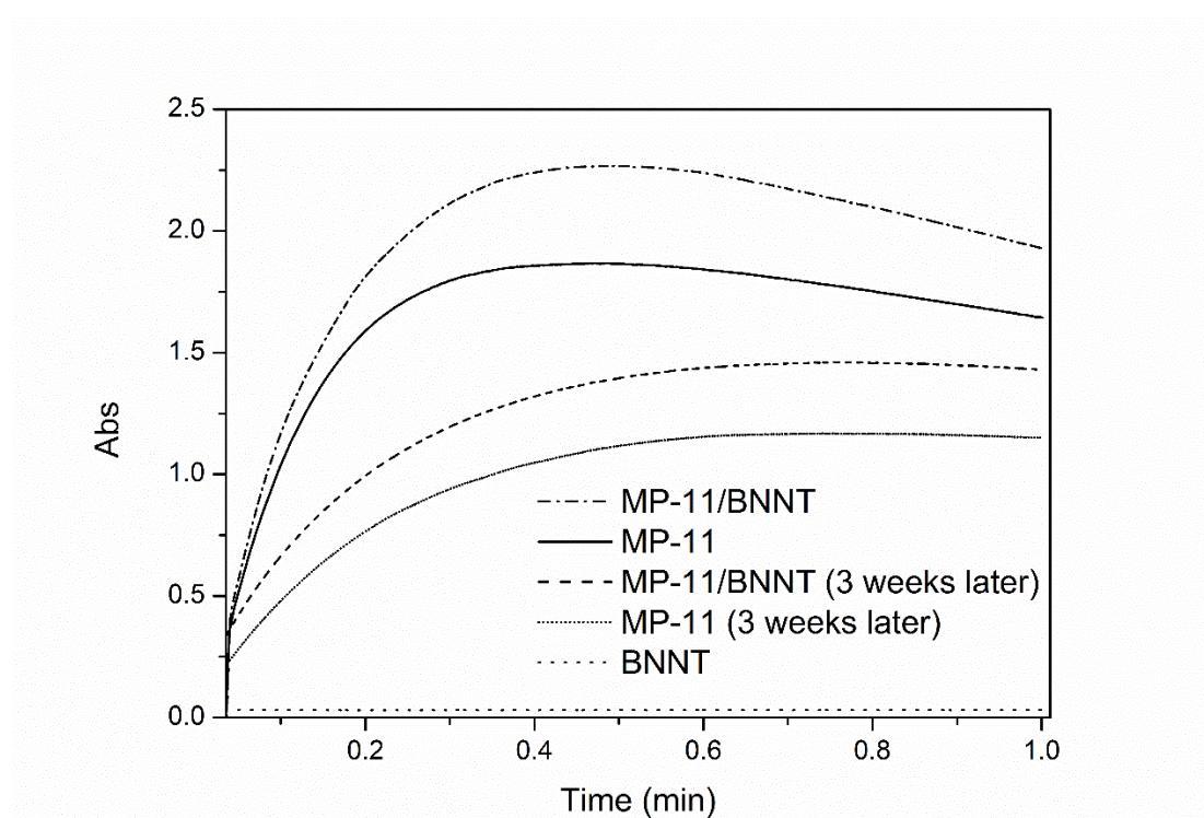
**Fig. S7** Monitored the reactions by kinetics mode at 652 nm using UV-vis spectrometer; the stability of the catalysts with various time have been preliminarily examined: The top two lines represent the samples left overnight at room temperature just after self-assembly of MP-11 on BNNTs, the next group have been stored at 4°C to maintain the stability for three weeks for investigation.
