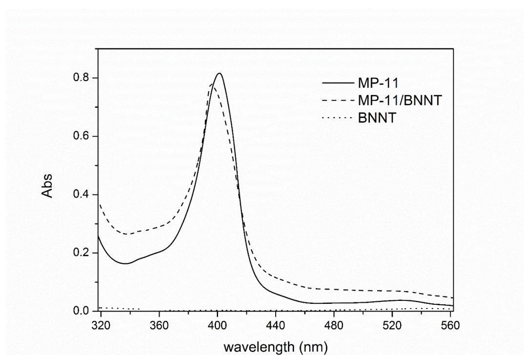
**Fig. S3** UV-visible spectrum of MP-11 coated BNNT. The solid, dotted and dashed lines represented the absorbance of pure MP-11 BNNT, and MP-11/BNNT respectively. After coating with MP-11, the soiret band at 405 nm shift to 396 nm, indicating  $\pi$ - $\pi$  stacking interactions between MP-11 and BNNTs.
