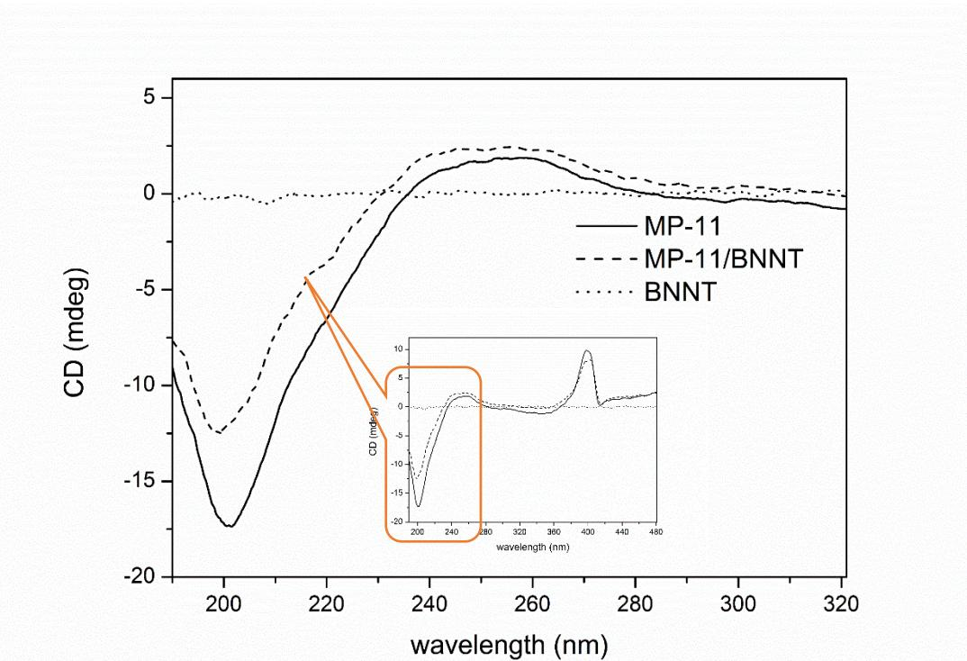
**Fig. S4** The CD spectrum of MP-11, BNNT and MP-11/BNNT. The negative band at 203 nm was shifted to 197 nm, indicating the secondary structure of MP-11 molecules was changed after coating with BNNTs.
