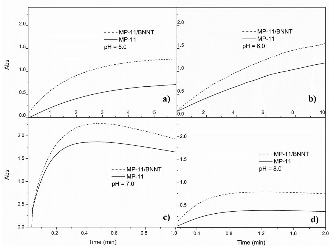
**Fig. S6** The plots of absorbance against time at different pH conditions, used to monitor the reactions by kinetics mode at 652 nm using UV-vis spectrometer; the stability of the catalysts in the diverse pH conditions have been investigated; a), b), c) and d) stand for pH 5.0, 6.0, 7.0 and 8.0, respectively; highest value of absorbance was found in pH 7.0, indicating reaction would be the most efficient when catalyzed by MP-11 /BNNTs nanohybrids at this pH condition.
