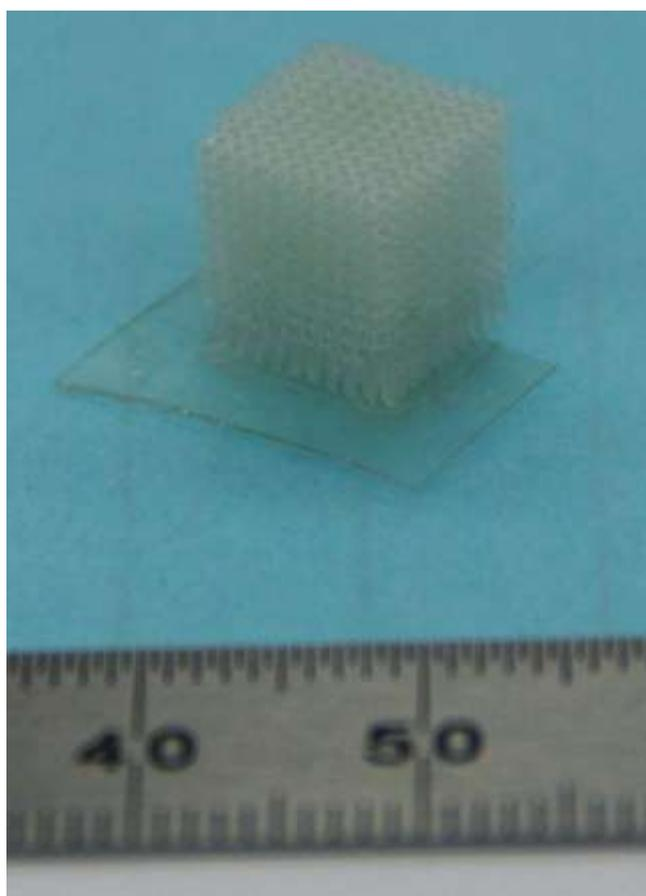
**Fig. S1.** Photograph of 3D printed *iLattice*.
