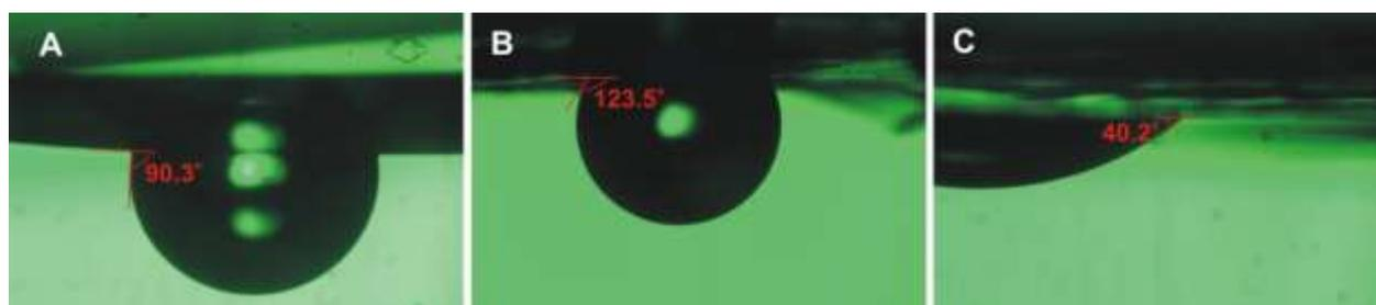
**Fig. S2.** Water contact angle of 3D printed flat film using 5 wt% BrMA customized resin before (A) and after poly(PFMA) (B) and poly(PEGMA) (C) grafting via SI-ATRP.
