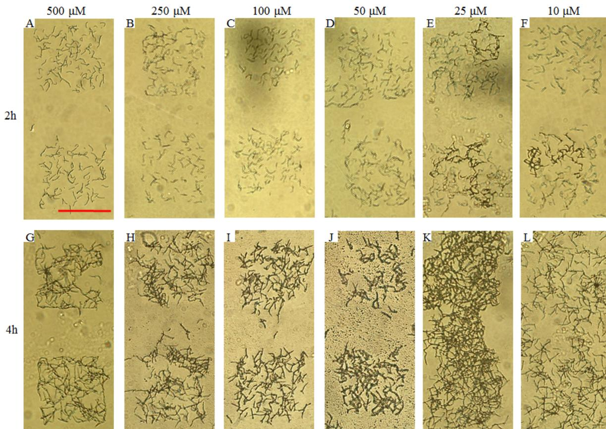
**S5.** Optical micrograph images taken at 2h (A to F) and 4h (G to L) for adhesion of *C. albicans* hyphae in RPMI1640 containing cyclic peptide (RGDFK), on 380  $\mu\text{m}$ -wide square patterns of pentadecane thiol, surrounded by bioinert SAMs containing immobilized tripeptide sequence of N'-AGRGDSC-C'. Scale bar = 380  $\mu\text{m}$ .
