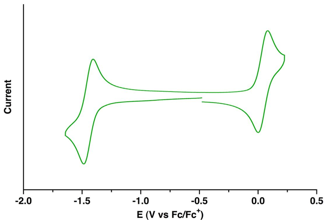
Figure S2. Cyclic voltammogram of Pt(HexylTIDS)(PPh<sub>3</sub>)<sub>2</sub>.
