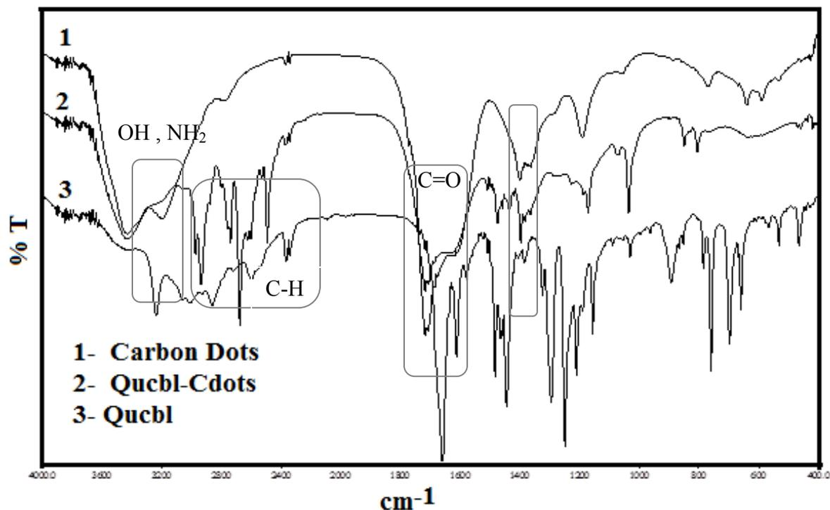
**Figure S5:** Overlay FT-IR spectra of Carbon dots (Cdots), Quinclorambucil(Quinclorambucil) and Quinclorambucil loaded carbon dots(Quinclorambucil-Cdots).
