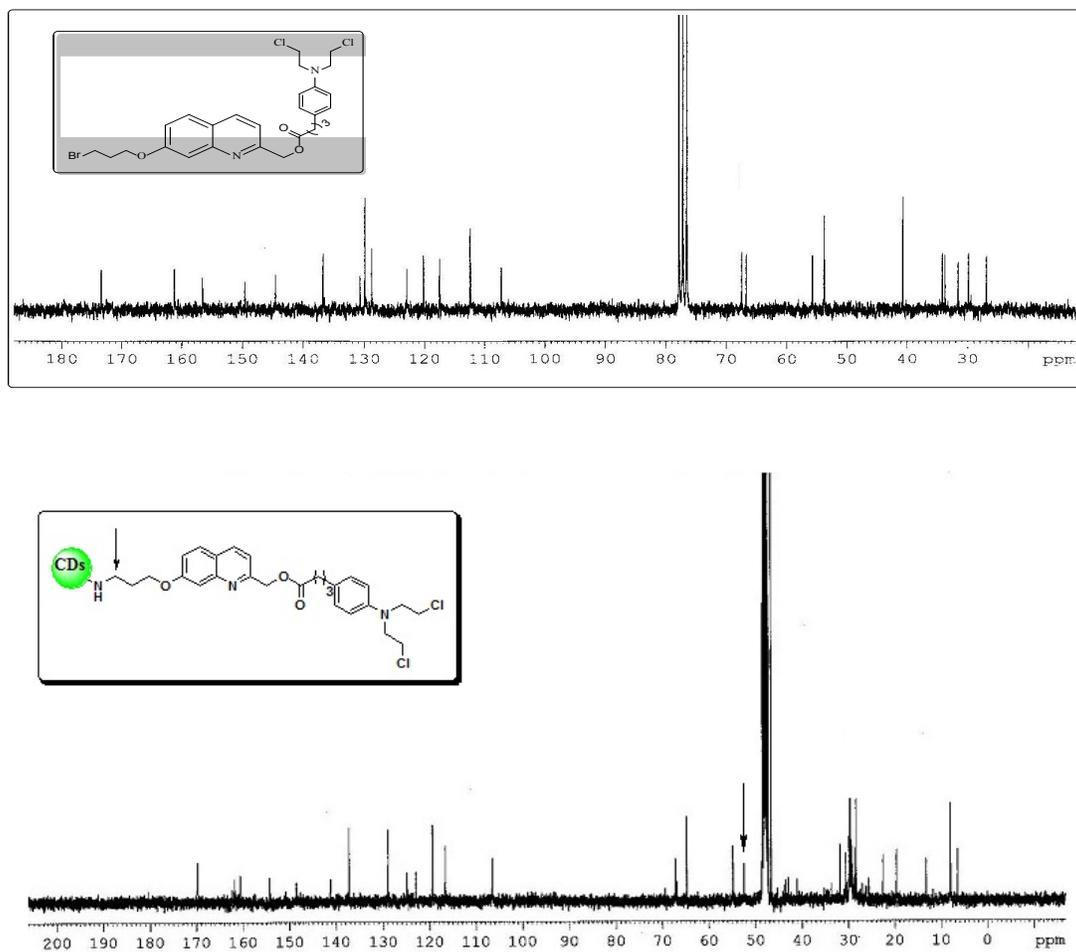
Figure S6:  $^{13}\text{C}$  NMR spectra of Cdots and Qucbl-Cdots in 100 MHz
