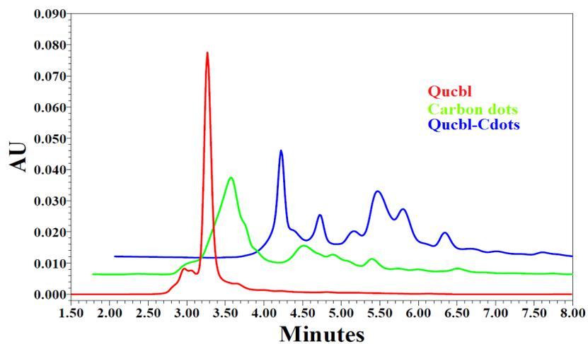
**Figure S7:** Overlay HPLC profile of Quinoline chlormbucil, Carbon dots and Quinoline chlorambucil loaded carbon dots in reverse phase HPLC using methanol/ water (8:2 v/v), at a flow rate of 1 mL / min.
