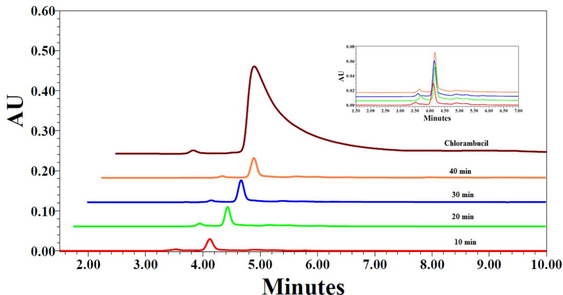
**Figure S14a:** HPLC profile of Chlorambucil release from Qucbl-Cdots using Red laser. The *y*-axes were offset by 40 mAU units and the *x*-axes were offset by 10 s, to facilitate better visualization.
