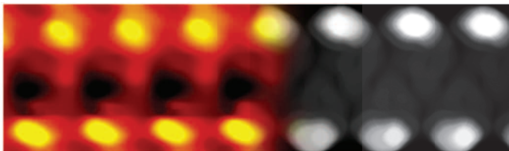
Figure S5. The ribbon structure of BBA molecule shown in Figure 2b (left panel) overlaid with the corresponding STM image simulation (right panel) in the bias condition of 1.05 V which is consistent with the experimental condition.
