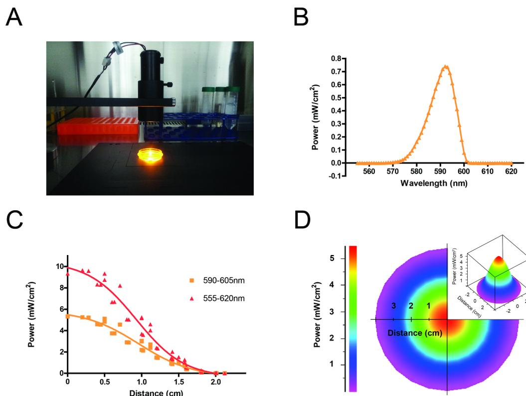
**Figure S5.** LED-based LIS and dosimetry. (A) Photograph of the LED-based LIS. (B) Wavelength- dependent power spectrum of the LED light. (C-D) Distance-power map of the LED-based LIS.
