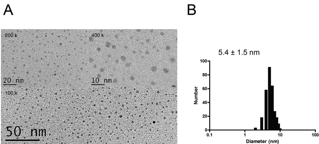
**Figure S3.** TEM images and measured sizes of the micelles with the non-staining method.
