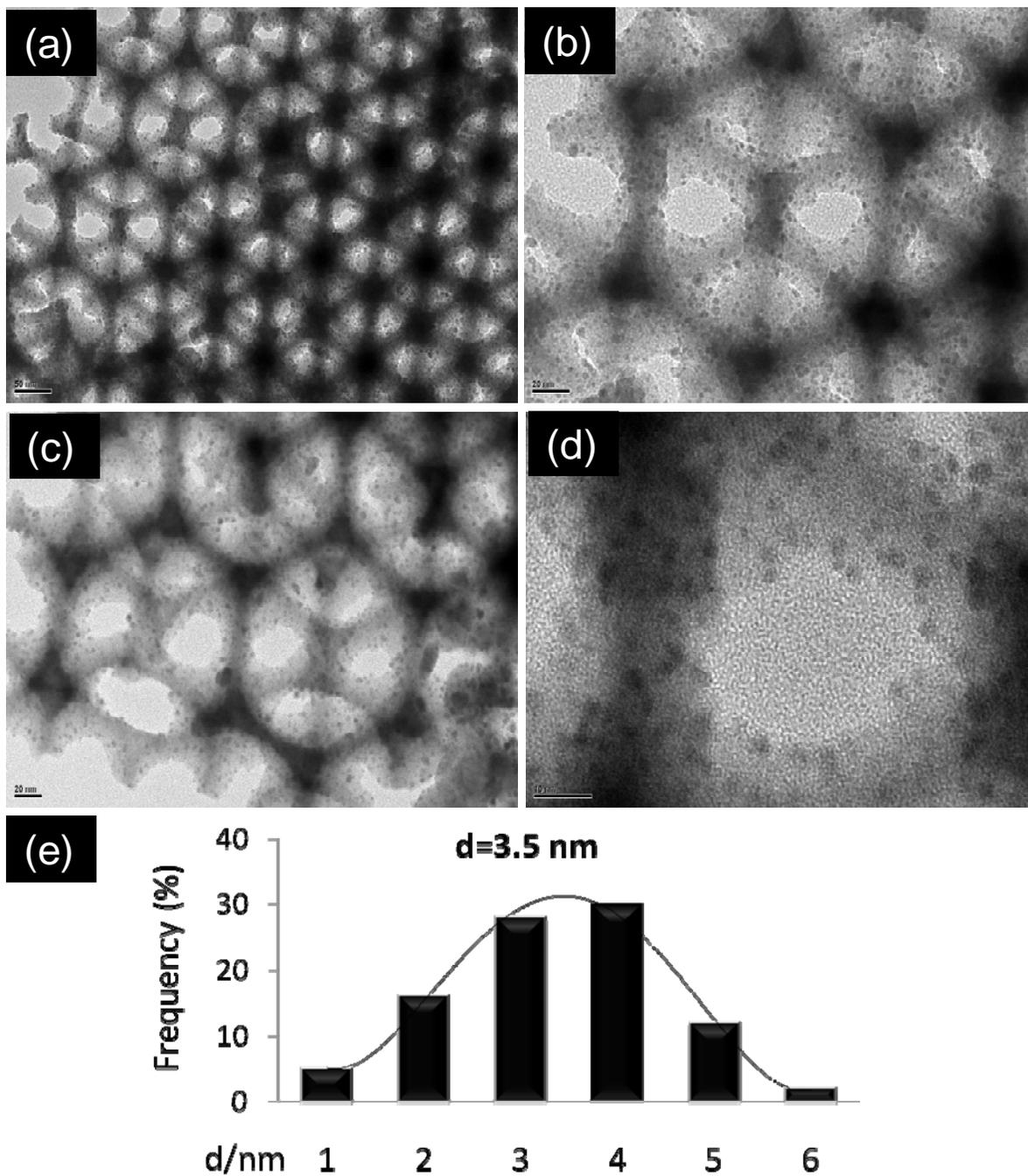
**Fig. S6** TEM (a-c) and HRTEM (d) images and size distribution (e) of Ag NPs by statistic analysis of more than 200 Ag particles in HRTEM images of 5.71 wt% Ag/3DOM  $\text{La}_{0.6}\text{Sr}_{0.4}\text{MnO}_3$ .
