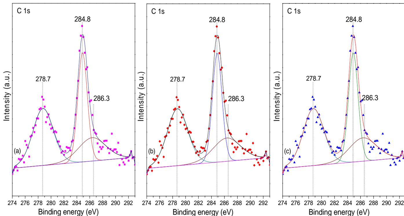
**Fig. S7.** C 1s XPS spectra of (a) 1.58 wt% Ag/3DOM  $\text{La}_{0.6}\text{Sr}_{0.4}\text{MnO}_3$ , (b) 3.63 wt% Ag/3DOM  $\text{La}_{0.6}\text{Sr}_{0.4}\text{MnO}_3$ , and (c) 5.71 wt% Ag/3DOM  $\text{La}_{0.6}\text{Sr}_{0.4}\text{MnO}_3$ .
