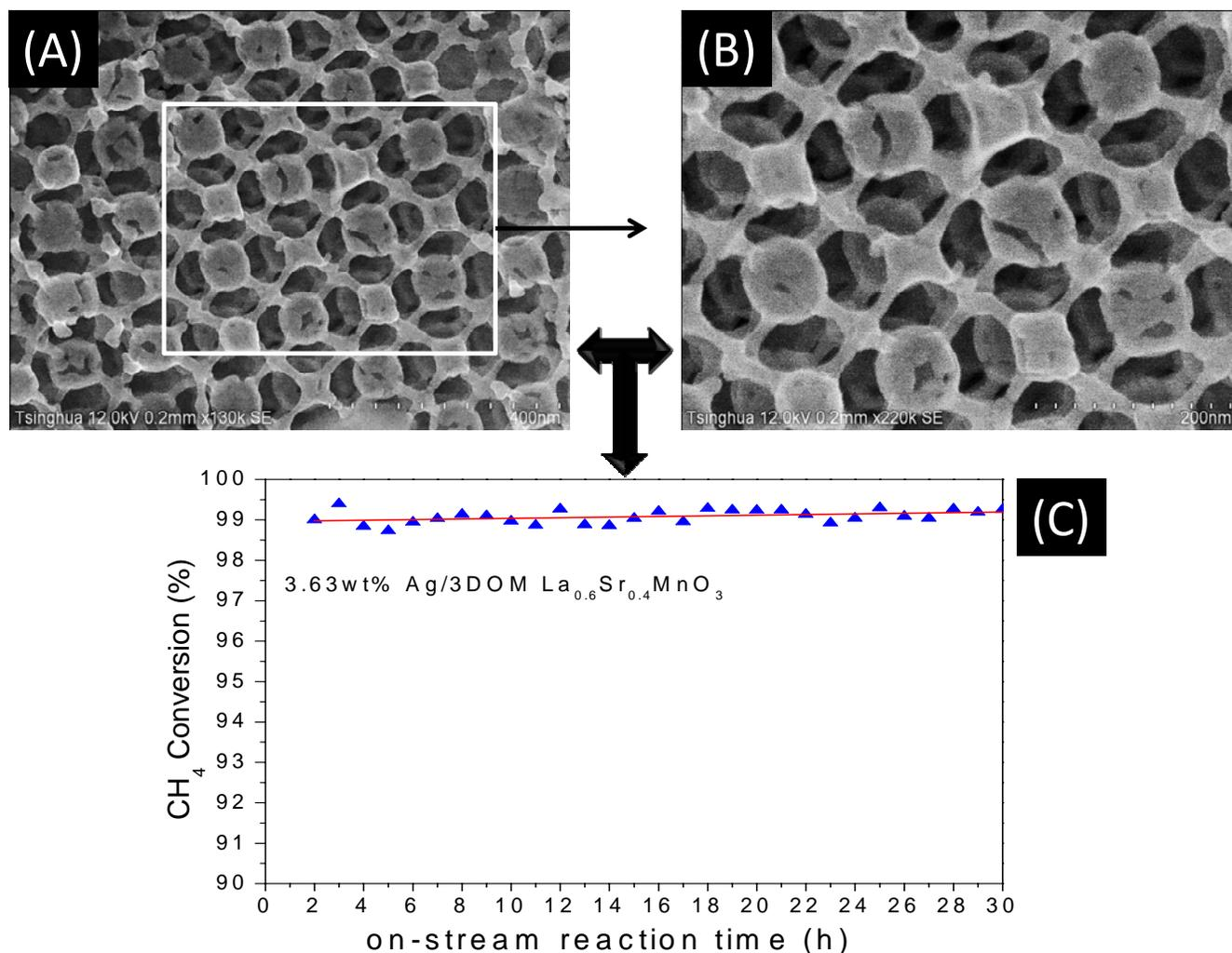
**Fig. S8.** (A, B) SEM image of 3.63 wt% Ag/3DOM La<sub>0.6</sub>Sr<sub>0.4</sub>MnO<sub>3</sub> after 30 h of on-stream reaction under the conditions of 2% CH<sub>4</sub> + 20% O<sub>2</sub> + 78% N<sub>2</sub> (balance) and GHSV = 30,000 mL/(g h).
