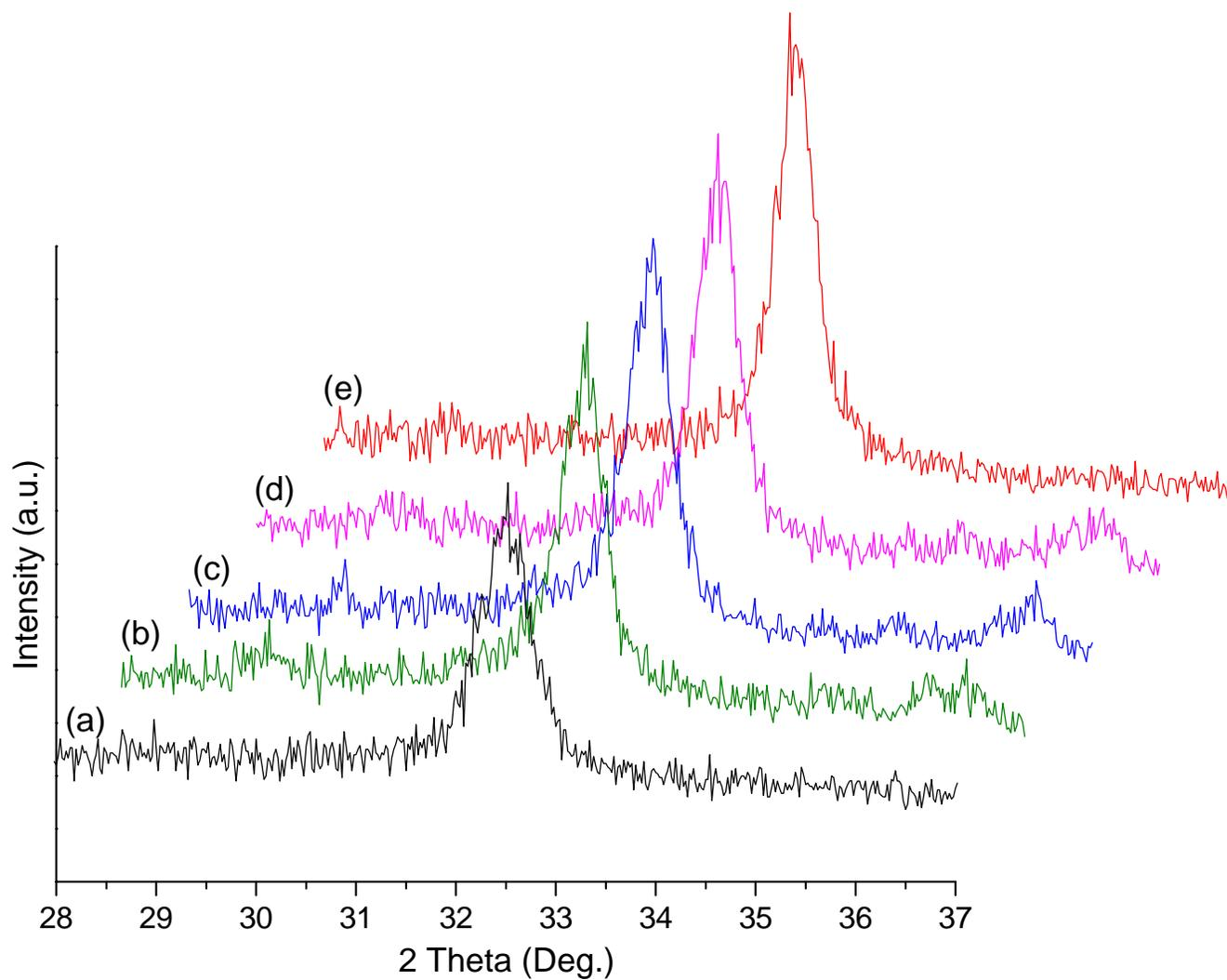
**Fig. S2.** Evolution of the XRD highest peak of (a) Bulk  $\text{La}_{0.6}\text{Sr}_{0.4}\text{MnO}_3$ , (b) 3DOM  $\text{La}_{0.6}\text{Sr}_{0.4}\text{MnO}_3$ , (c) 1.58 wt% Ag/3DOM  $\text{La}_{0.6}\text{Sr}_{0.4}\text{MnO}_3$ , (d) 3.63 wt% Ag/3DOM  $\text{La}_{0.6}\text{Sr}_{0.4}\text{MnO}_3$ , and (e) 5.71 wt% Ag/3DOM  $\text{La}_{0.6}\text{Sr}_{0.4}\text{MnO}_3$ .
