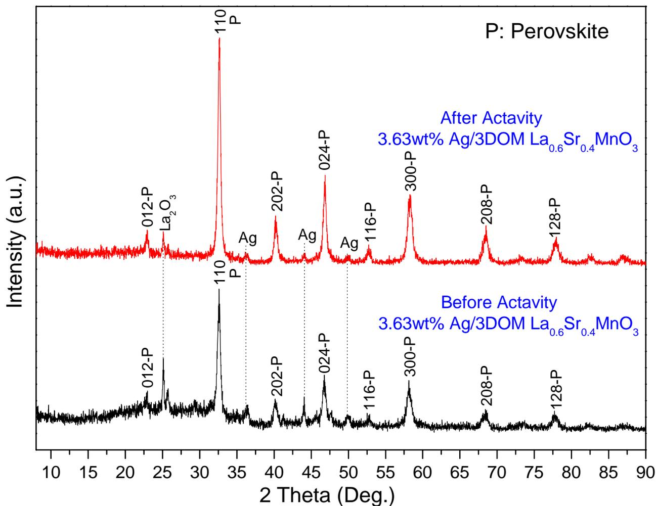
**Fig. S9.** XRD pattern of the 3.63 wt% Ag/3DOM La<sub>0.6</sub>Sr<sub>0.4</sub>MnO<sub>3</sub> sample after 20 h of on-stream reaction at GHSV = 30,000 mL/(g h).
