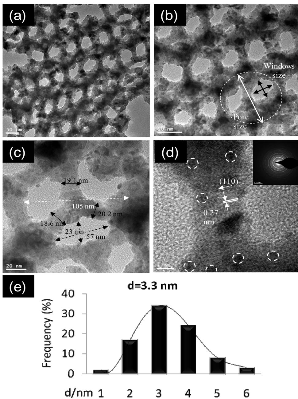
**Fig. S4** TEM images (a, b) and HRTEM images (c, d) and size distribution of Ag NPs (e) of 1.58 wt% Ag/3DOM  $\text{La}_{0.6}\text{Sr}_{0.4}\text{MnO}_3$ .
