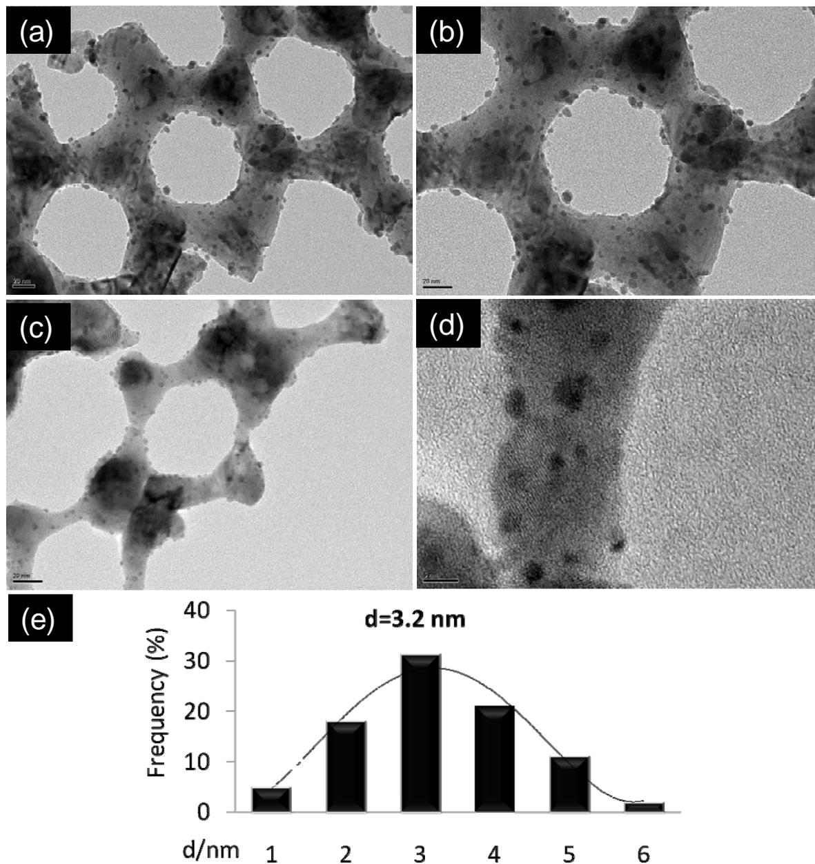
**Fig. S5** (a-c) TEM and (d) HRTEM images and size distribution (e) of Ag NPs by statistic analysis of more than 200 Ag particles in HRTEM images of 3.63 wt% Ag/3DOM  $\text{La}_{0.6}\text{Sr}_{0.4}\text{MnO}_3$ .
