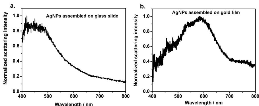
**Figure S9** (a) normalized scattering spectrum of 100 nm AgNPs assembled on glass slide. (b) normalized scattering spectrum of 100 nm AgNPs assembled on gold film.
