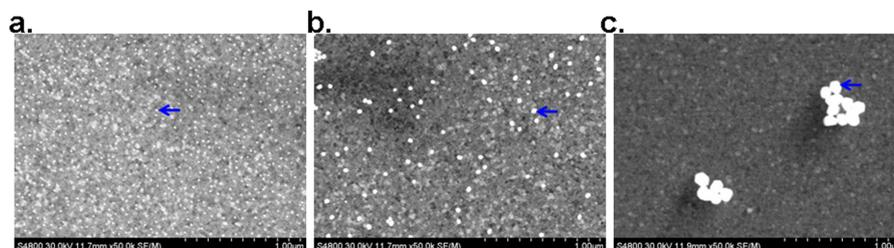
**Figure S5.** SEM images of (a) 14 nm, (b) 40 nm and (c) 120 nm gold nanoparticles. Arrows point to gold nanoparticles.
