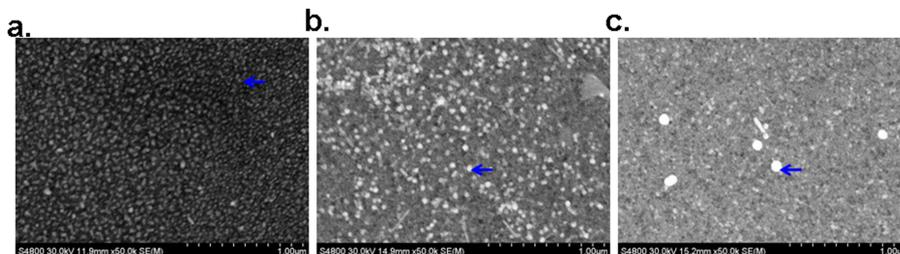
**Figure S4.** SEM images of (a) 20 nm, (b) 50 nm and (c) 100 nm silver nanoparticles. Arrows point to silver nanoparticles
