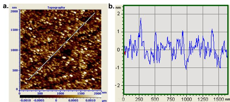
**Figure S1.** (a) AFM image of gold substrate (b) Depth analysis of the area shown in part (a) indicated by line.
