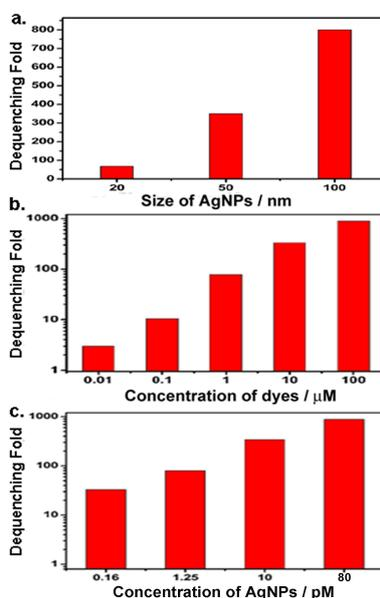
**Figure S3** (a) SPCE dequenching folds responding to sizes of adsorbed silver nanoparticles (AgNPs). (b) SPCE dequenching folds responding to the concentrations of dyes added on the gold film. 100 nm AgNPs were used. (c) SPCE dequenching folds responding to the concentrations of AgNPs added onto the surface. The concentrations of dyes were 100  $\mu\text{M}$ .
