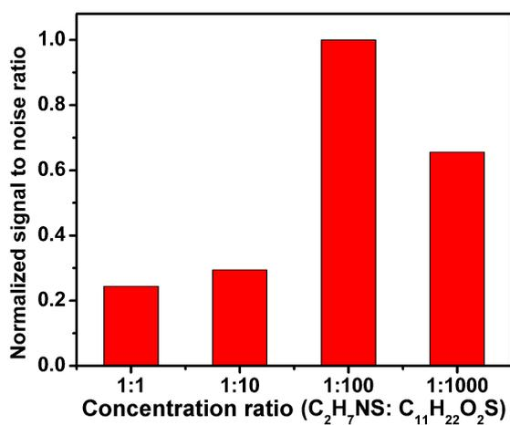
**Figure S10.** The normalized signal to noise ratio responding to different concentration ratio of cysteamine (100  $\mu$ M) to 11-Mercaptoundecanoic acid used to modify the gold surface.
