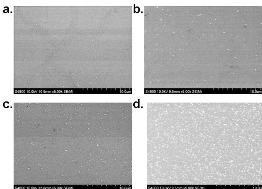
**Figure S8.** (a) 0.16 pM, (b) 1.25 pM, (c) 10 pM and (d) 80 pM 100 nm silver nanoparticles added to gold surface to form NPs-Film structure tested by SEM image.
