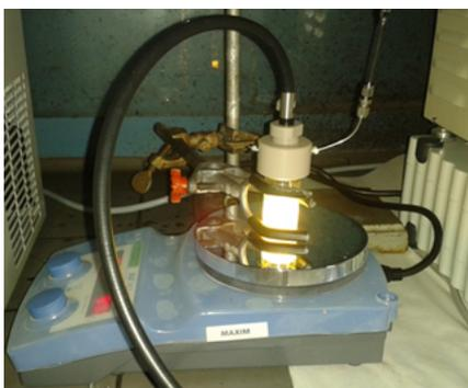
**Figure S2. Photocatalytic reactor at work**
