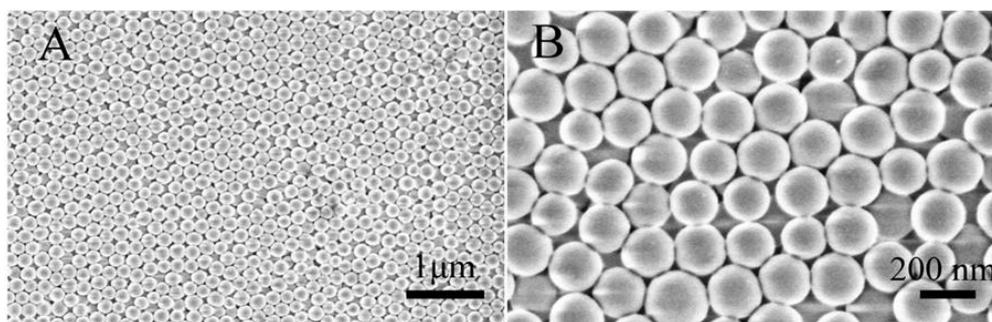
Fig. S1 SEM images (A and B) with different magnification of the colloidal SiO<sub>2</sub> spheres prepared via classical the St öber method.
