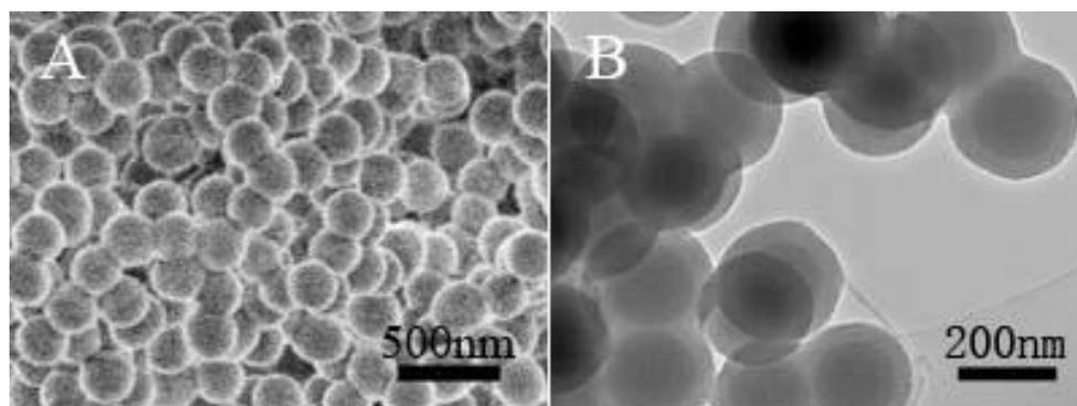
Fig. S2 FESEM (A) and TEM (B) images of the core-shell  $\text{SiO}_2@RF$  nanospheres prepared via a modified St öber coating method.
