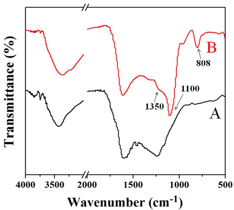
Fig. S7 FTIR spectrum of the hollow carbon nanospheres with(B) and without (A) nitrogen doping.
