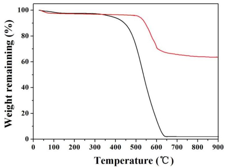
Fig. S3 TG curve of the N-HCS in air (black) and N<sub>2</sub> (red) atmospheres with a heating rate of 5 °C /min from 25 to 700 °C.
