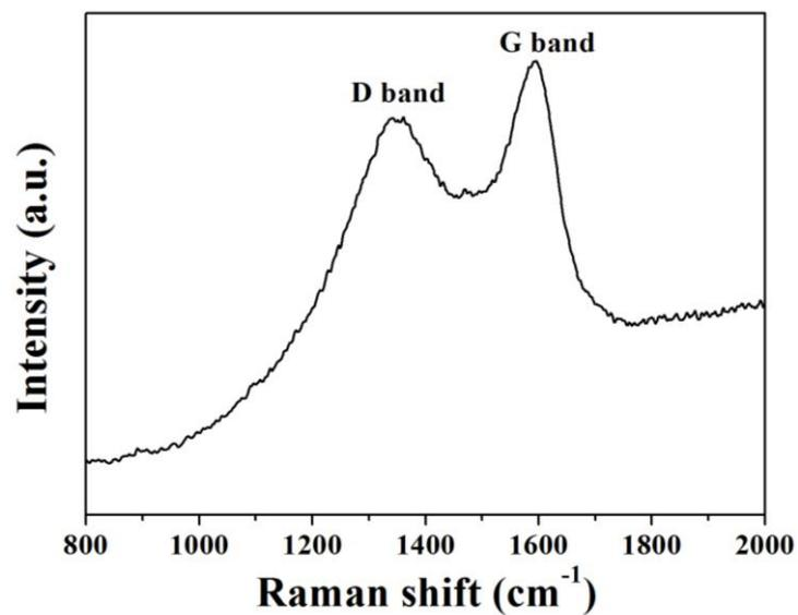
Fig S8 Raman spectra of the nitrogen-doped hollow carbon nanospheres. The ratio of peak intensity ( $I_D/I_G$ ) is 0.96.
