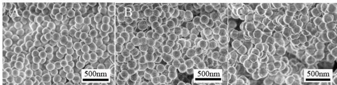
Fig. S4 FESEM images of the core-shell  $\text{SiO}_2$ @N-CS spheres synthesized with different resorcinol concentrations: (A) 0.0885; (B) 0.118; (C) 0.236 mol/L.
