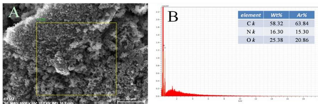
Fig. S6 (A) Typical SEM image of N-HCSs via a two-step St öber method followed by the carbonization with melamine and the removal of the silica cores and (B) EDX spectra show the chemical composition of the areas labeled by the yellow square.
