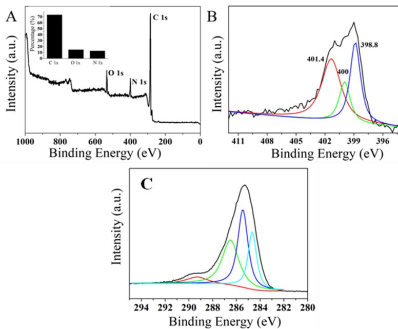
Fig. S5 X-ray photoelectron spectra (XPS) of the N-HCS spheres prepared via a two-step St öber method followed by the carbonization with melamine and the removal of cores: A) the survey spectrum; B) N<sub>1s</sub> and C) high-resolution spectra of C<sub>1s</sub>. The insert in A is the corresponding content of each element.
