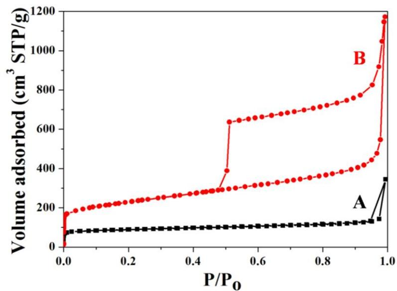
Fig. S9 N<sub>2</sub> sorption isotherms of the core-shell SiO<sub>2</sub>@nitrogen-doped carbon nanospheres (SiO<sub>2</sub>@N-CSs) (A) and N-doped hollow carbon spheres (N-HCSs) (B).
