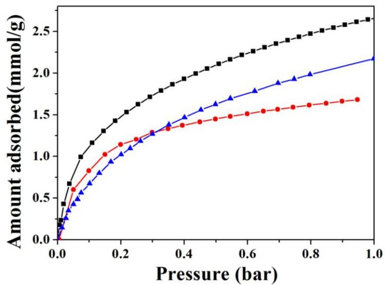
Fig S10 CO<sub>2</sub> adsorption isotherms of the N-HCSs with different N content: 3.1 wt% (red), 6.7 wt% (blue), and 14.8 wt% (black) at 298 K and 1.0 bar.
