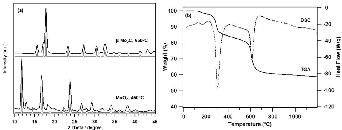
**Figure S3.** (a) XRD patterns of the post-calcined sample at 450°C and at 650°C, at the *o*-phenylenediamine: Mo=2:1, (b) TGA/DSC curves for *o*-phenylenediamine/ $(\text{NH}_4)_6\text{Mo}_7\text{O}_{24}$  system.
