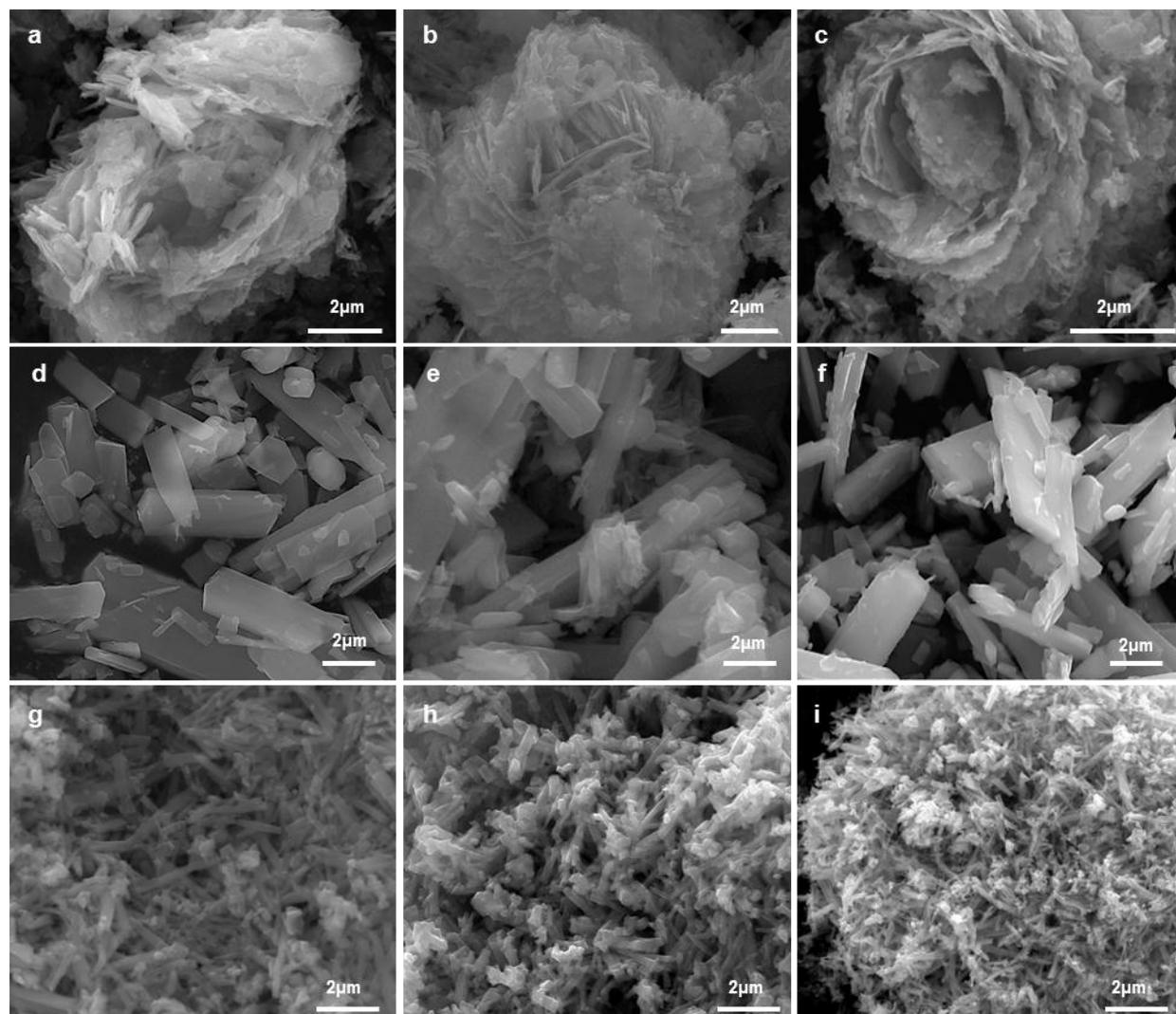
Figure S4. SEM images of the micro-flowers synthesized by 4-Cl-*o*-phenylenediamine at (a) 350°C, (b) 450°C, and (c) 675°C, the flake-like particles synthesized by *o*-phenylenediamine at (d) 350°C, (e) 450°C, and (f) 625°C, and the nano-rods synthesized by 2-nitro-*p*-phenylenediamine at (g) 350°C, (h) 450°C, and (i) 875°C. The molar ratio of amine: Mo=2:1.
