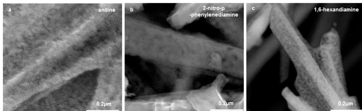
**Figure S1.** High resolution SEM images of porous  $\beta$ - $\text{Mo}_2\text{C}$  nano-particles synthesized by (a) aniline, at  $675^\circ\text{C}$ , (b) 2-nitro-*p*-phenylenediamine, at  $875^\circ\text{C}$ , (c) 1,6-hexanediamine, at  $675^\circ\text{C}$ .
