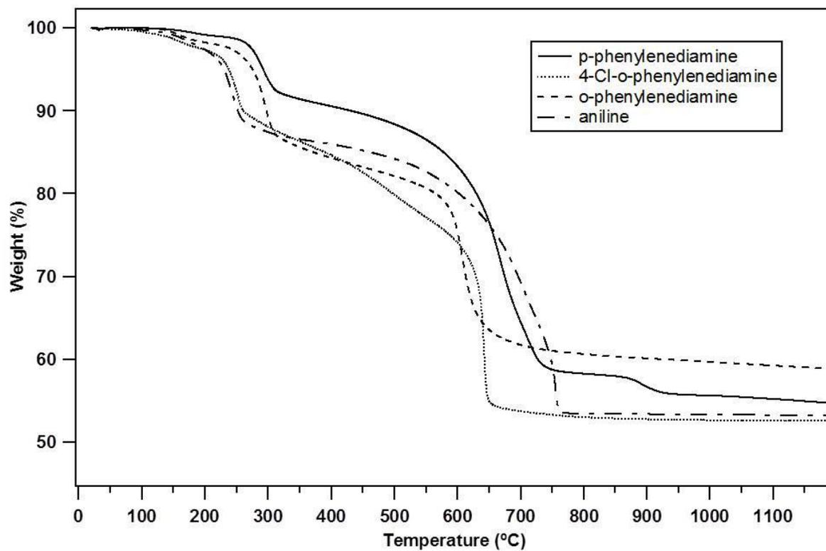
**Figure S5.** TGA curves for (a) *o*-phenylenediamine/ $(\text{NH}_4)_6\text{Mo}_7\text{O}_{24}$  system, (b) *p*-phenylenediamine/ $(\text{NH}_4)_6\text{Mo}_7\text{O}_{24}$  system, (c) aniline/ $(\text{NH}_4)_6\text{Mo}_7\text{O}_{24}$  system, (d) 4-Cl-*o*-phenylenediamine/ $(\text{NH}_4)_6\text{Mo}_7\text{O}_{24}$  system, at amine: Mo=2:1
