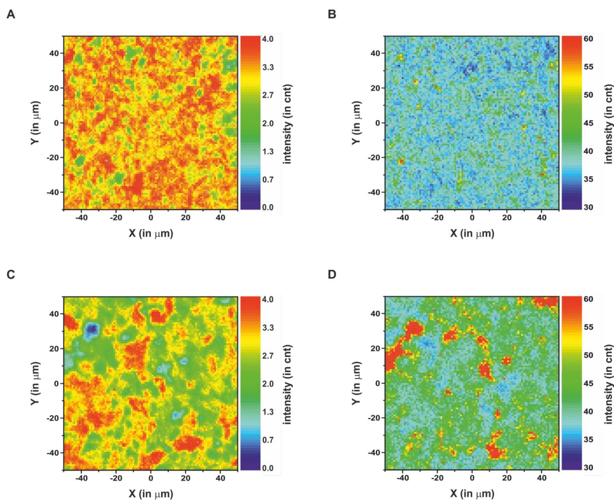
**Figure S4:** Raman maps of dodecyl-functionalized graphene samples:  $\lambda_{\text{exc.}} = 532 \text{ nm}$ ,  $10,000 \mu\text{m}^2$ ; A) Mean  $I_D/I_G$  ratio of  $\text{C}_{12}\text{H}_{25}\text{-G}(\text{powder})$  and B) FWHM of the respective 2D-band, C) Mean  $I_D/I_G$  ratio of  $\text{C}_{12}\text{H}_{25}\text{-G}(\text{spherical})$  and D) FWHM of the respective 2D-band.
