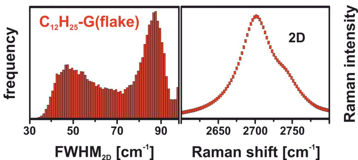
**Figure S6:** Left: Raman histogram (FWHM<sub>2D</sub>) of the dodecyl-functionalized flake graphite.
