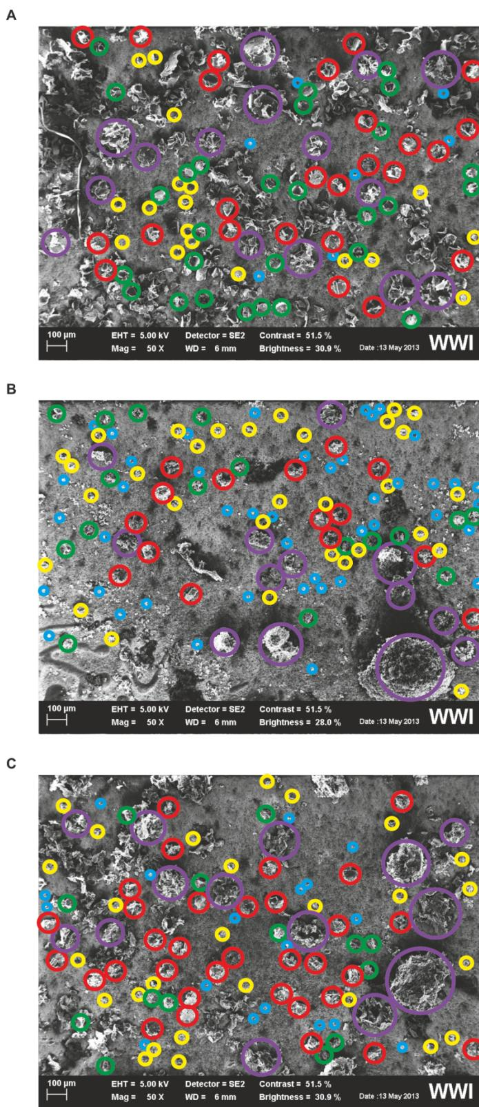
**Figure S1:** SEM images of A)  $\text{C}_{12}\text{H}_{25}\text{-G}(\text{flake})$ , B)  $\text{C}_{12}\text{H}_{25}\text{-G}(\text{powder})$  and C)  $\text{C}_{12}\text{H}_{25}\text{-G}(\text{spherical})$  for the determination of the grain size (see Table S4).
