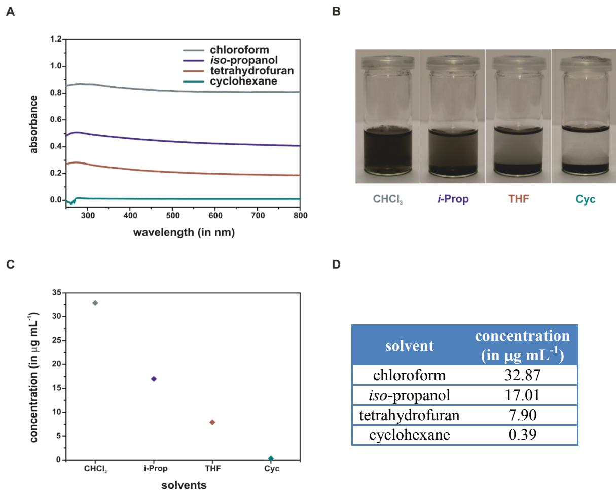
**Figure S8:** A) UV/vis spectra of dodecyl-functionalized powder graphite in different solvents (chloroform, *iso*-propanol, tetrahydrofuran, cyclohexane), B) correspondent dispersions and C), D) calculated concentrations.
