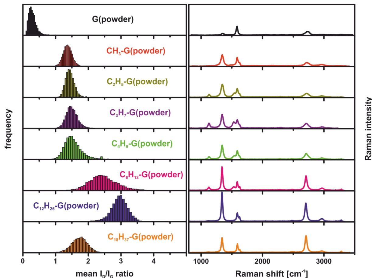
**Figure S5:** Raman histograms ( $I_D/I_G$ -ratio) and averaged Raman spectra (10,000 single point spectra) of the starting graphite (black) and the alkyl-functionalized materials (colour coded),  $\lambda_{\text{exc.}} = 532 \text{ nm}$  - spectra normalized to G-band intensity.
