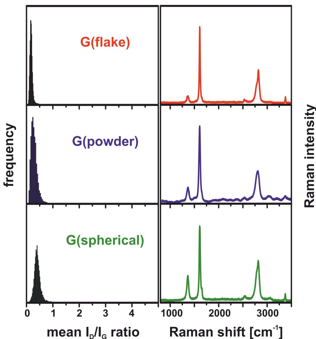
**Figure S3:** Raman histograms ( $I_D/I_G$ -ratio) and averaged Raman spectra (10,000 single point spectra) of the starting graphites,  $\lambda_{\text{exc.}} = 532$  nm - spectra normalized to G-band intensity.
