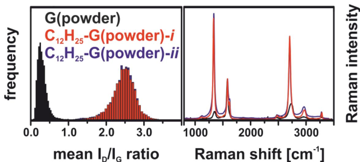
**Figure S2:** Left: Raman histograms ( $I_D/I_G$ -ratio) of the powder graphite (black) and two dodecyl-functionalized graphene samples (red and blue), prepared by the same procedure. Right: Correspondent averaged spectra (10,000 single point spectra) of the starting graphite and the functionalized materials,  $\lambda_{\text{exc.}} = 532 \text{ nm}$ .
