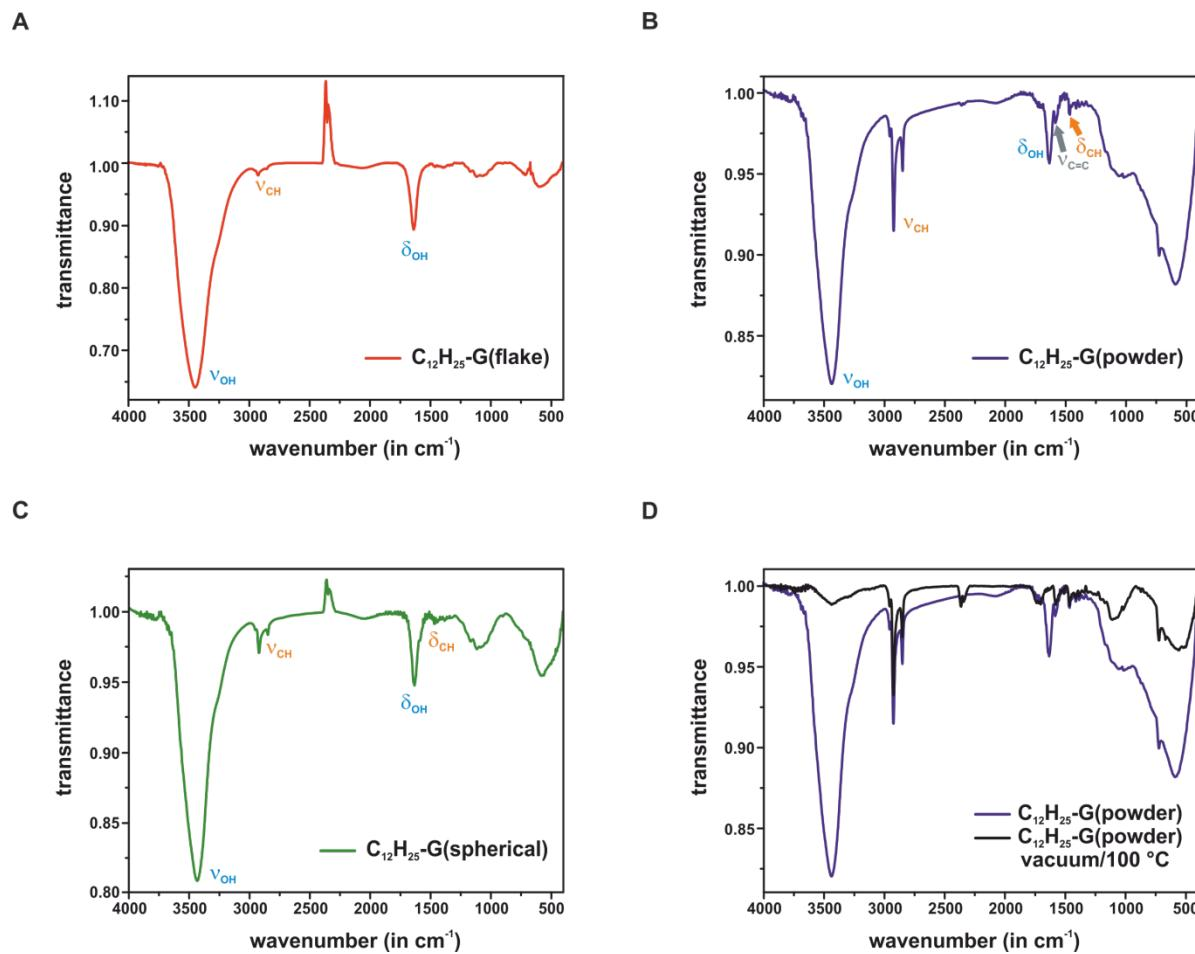
**Figure S7:** IR spectra of A)  $\text{C}_{12}\text{H}_{25}\text{-G}(\text{flake})$ , B)  $\text{C}_{12}\text{H}_{25}\text{-G}(\text{powder})$ , C)  $\text{C}_{12}\text{H}_{25}\text{-G}(\text{spherical})$  and D)  $\text{C}_{12}\text{H}_{25}\text{-G}(\text{powder})$  before and after heating the pellet at  $100\text{ }^\circ\text{C}$  in vacuum overnight.
