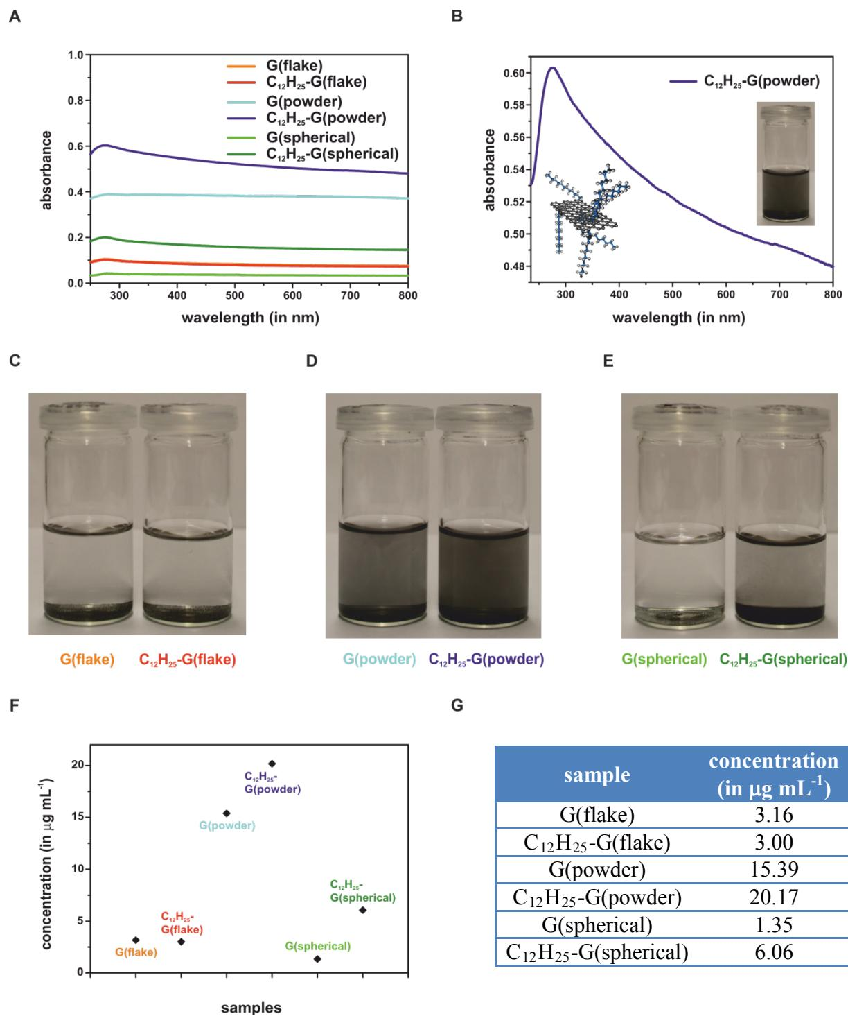
**Figure S9:** A) UV/vis spectra of pristine graphite and dodecyl-functionalized graphene, B) characteristic UV/vis spectrum of dodecyl-functionalized powder graphite and correspondent dispersions of pristine graphite (left) and dodecyl-functionalized graphene (right) in the case of C) flake graphite, D) powder graphite and E) spherical graphite and F), G) calculated concentrations.
