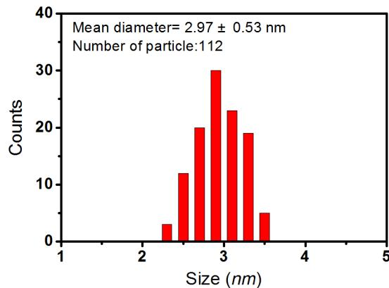
Figure S2. The corresponding HRTEM size histogram of Sv-Cu cluster. The data was obtained from 112 particles.
