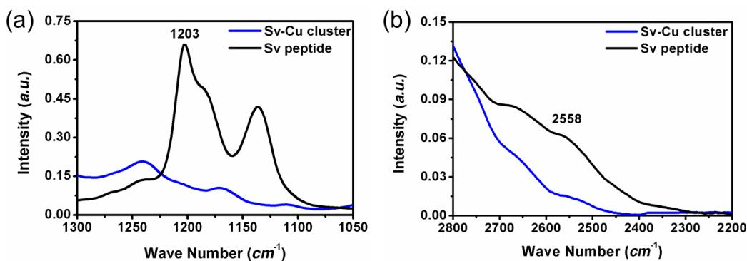
**Figure S1.** FTIR spectra of Sv peptide (black line) and Sv-Cu cluster (blue line). (a) and (b) the enlarged view of C-O-H vibration of Tyrosine and S-H vibration of cysteine, respectively.
