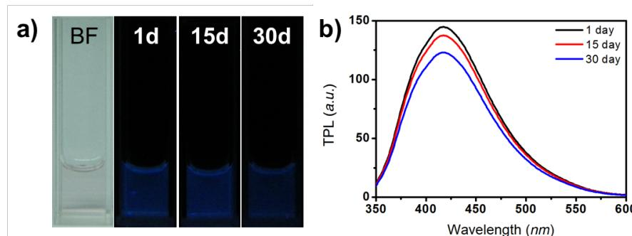
Figure S4. The physical stability of the Sv-Cu cluster probe solution. (a) Digital image of Sv-Cu cluster under room light and 365 nm UV light taken at different time (1d, 15d and 30d). (b) Time-followed fluorescence spectra of Sv-Cu cluster.
