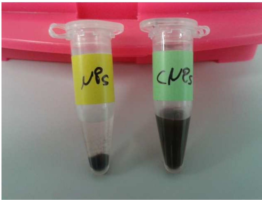
Fig. S1. Appearance of unmodified (NPs, yellow label) and citrate-stabilized magnetite nanoparticles (cNPs, green label) at concentrations of 3.5 mg/ml in water after 1 h of settling at RT under normal gravity. While magnetite nanoparticles showed strong precipitation, the negative surface charge of the citrate-coated nanoparticles (cNPs) ensure the presence of a colloidal solution.
