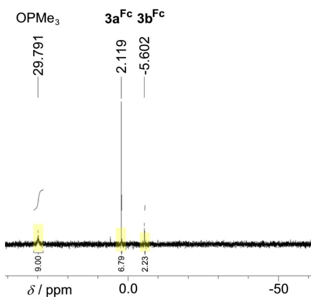
Fig. S13.  $^{31}\text{P}\{\text{H}\}$  NMR spectrum of  $[\mathbf{2}^{\text{Fc}}]^{2+}$  and  $\text{PMe}_3$  (exc.) in  $\text{CD}_3\text{CN}$ .
