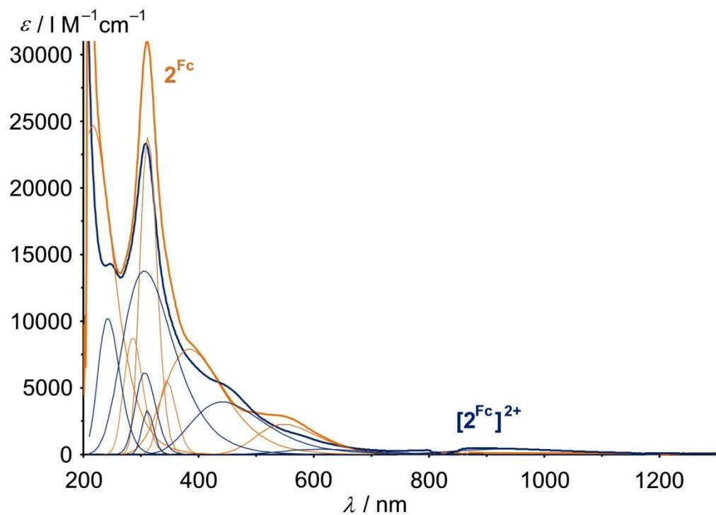
Fig. S9. Spectroelectrochemical oxidation of **2<sup>Fc</sup>** in THF/[<sup>n</sup>Bu<sub>4</sub>N][B(C<sub>6</sub>F<sub>5</sub>)<sub>4</sub>]; Pt electrodes; detector switch at 800 nm
