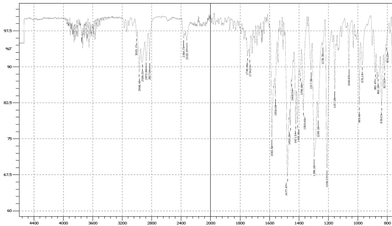
**Figure S 17** IR (ATR) spectrum for [Ir(cod)(*i*Pr)(OCO<sub>2</sub>Ph)] 13
