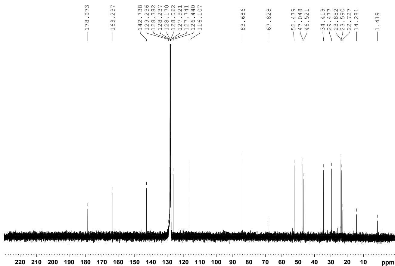
Figure S 23  $^{13}\text{C}\{\text{H}\}$  NMR (75 MHz,  $\text{C}_6\text{D}_6$ ) spectrum for  $[\text{Ir}(\text{cod})(\text{iPr})(\text{O}_2\text{CNHBn})]$  16
