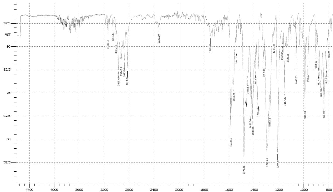
Figure S 9 IR (ATR) spectrum for  $[\text{Ir}(\text{cod})(\text{iPr})(\text{OPh})]$  11
