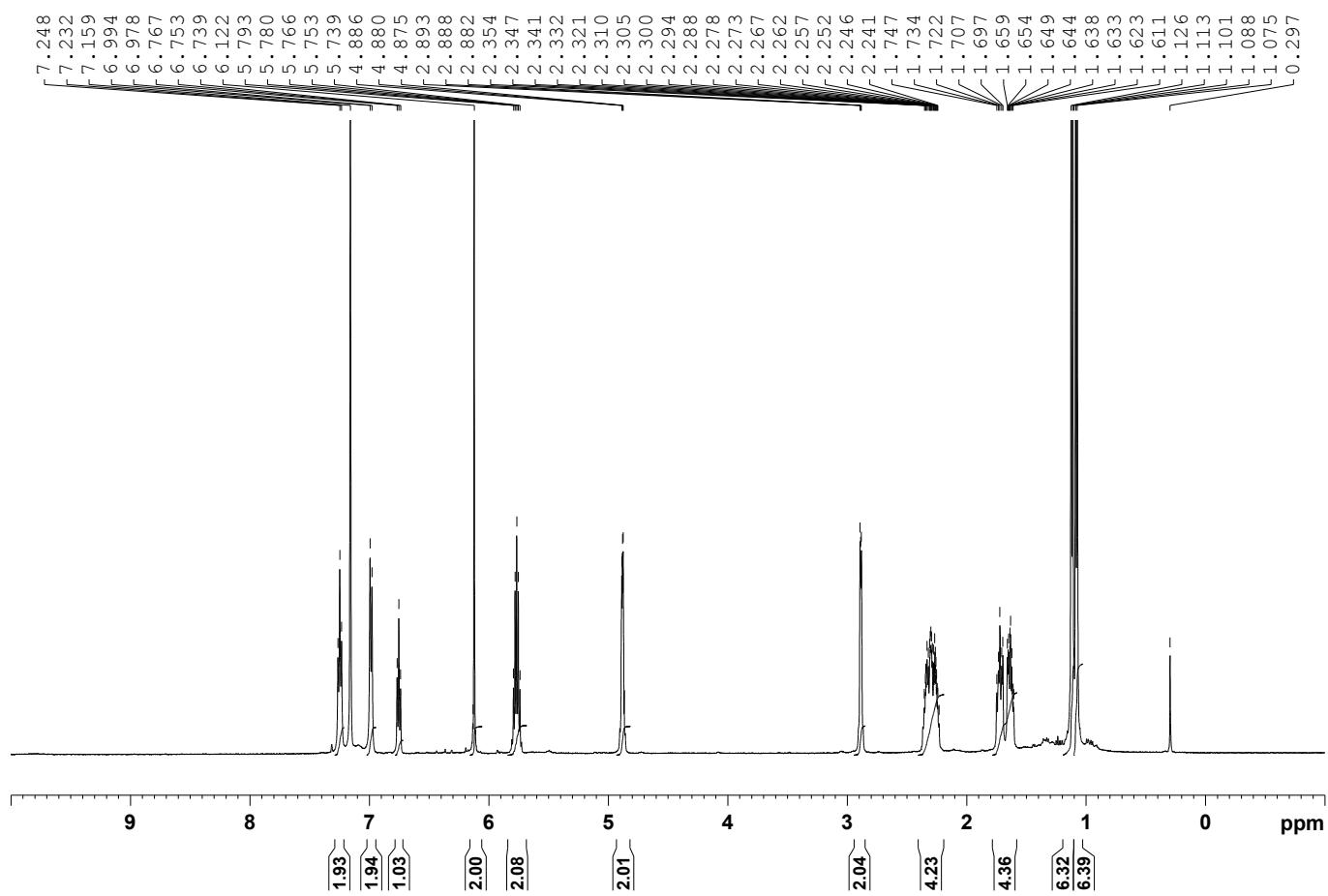
**Figure S 7**  $^1\text{H}$  NMR (300 MHz,  $\text{C}_6\text{D}_6$ ) spectrum for  $[\text{Ir}(\text{cod})(\text{iPr})(\text{OPh})]$  11
