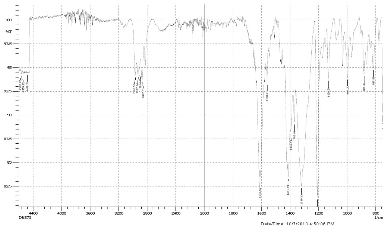
**Figure S 6** IR (ATR) spectrum for  $[\{\text{Ir}(\text{cod})(\text{I}^i\text{Pr})\}_2(\mu-\kappa^1:\kappa^2\text{-CO}_3)]$
