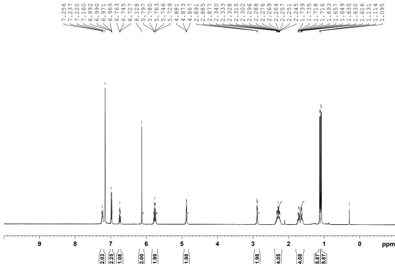
Figure S 14 <sup>1</sup>H NMR (300 MHz, C<sub>6</sub>D<sub>6</sub>) spectrum for  $[\text{Ir}(\text{cod})(\text{iPr})(\text{OCO}_2\text{Ph})]$  **13**
