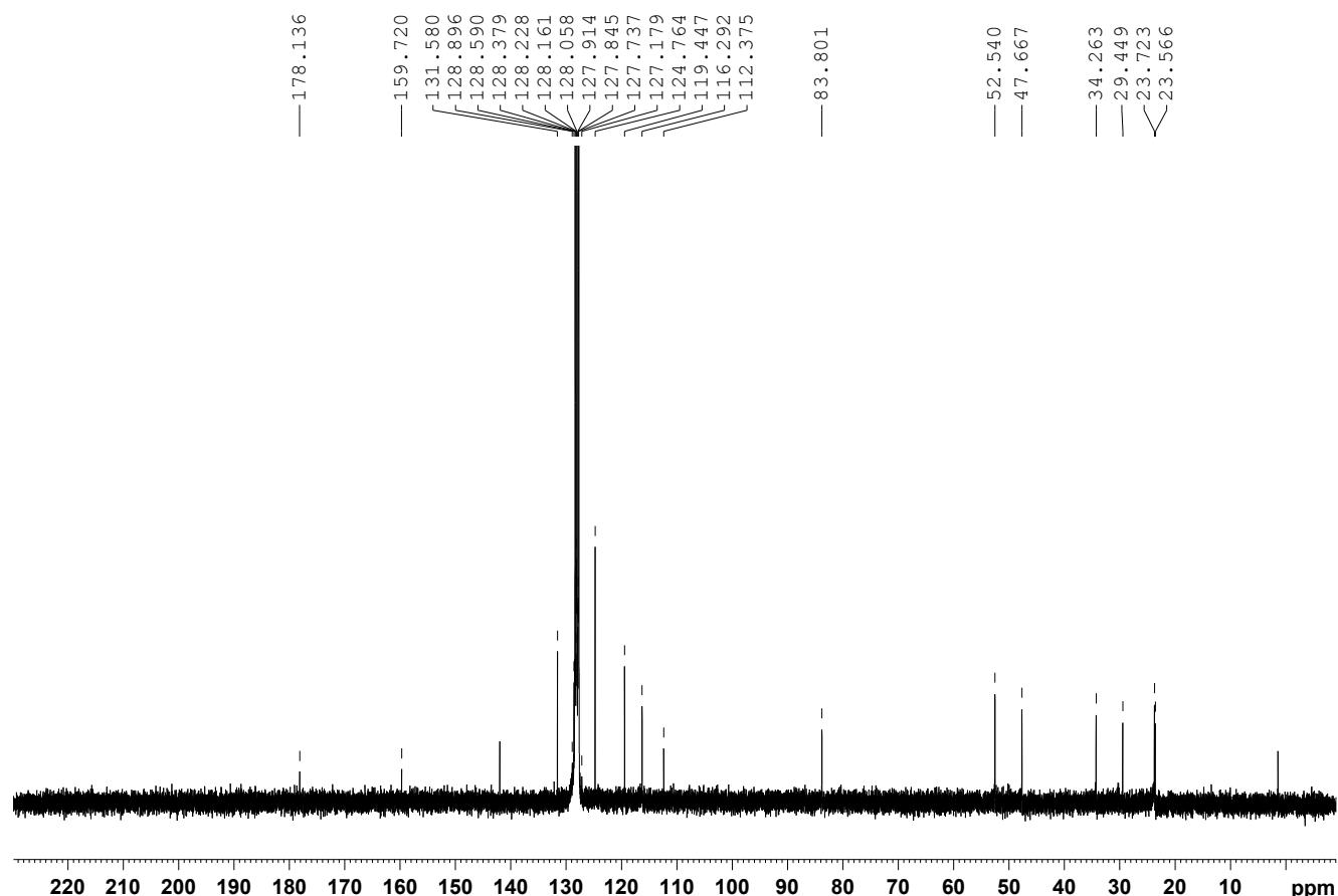
**Figure S 30** <sup>13</sup>C{<sup>1</sup>H} NMR (75 MHz, C<sub>6</sub>D<sub>6</sub>) spectrum for [Ir(cod)(iPr)(O<sub>2</sub>CNH(-*p*-BrC<sub>6</sub>H<sub>4</sub>))] **17**
