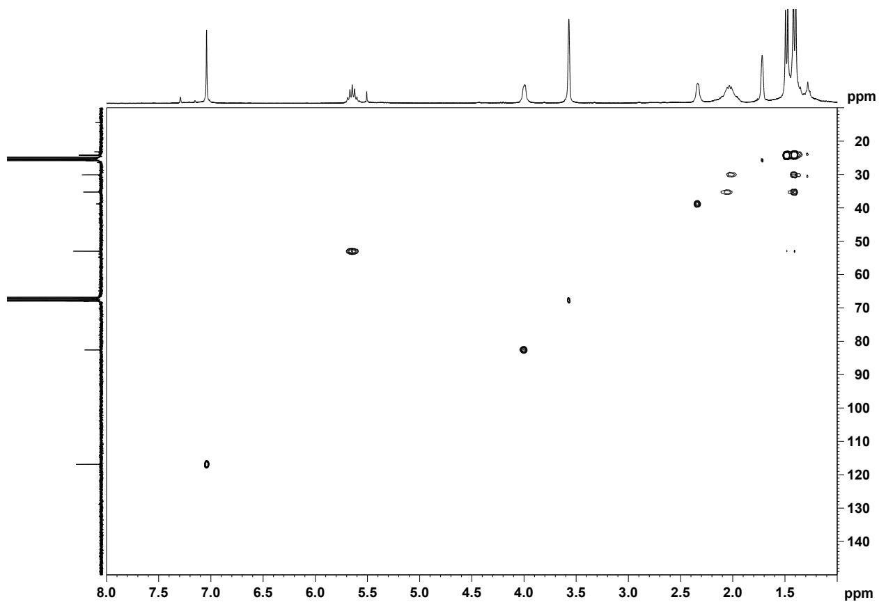
**Figure S 4** HSQC NMR (300 MHz, THF- $d_8$ ) spectrum for  $[\{\text{Ir}(\text{cod})(\text{iPr})\}_2(\mu-\kappa^1:\kappa^2-\text{CO}_3)]$  **8**
