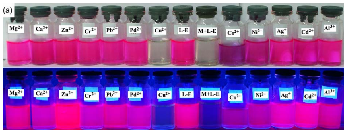
Fig. S7. Photographs (top: under room light; bottom: under 360 nm UV light; L = trans -SL; 1.0 \times 10^{-5} \text{ mol dm}^{-3} ; M+L = all the 18 metal ions+ trans -SL).
