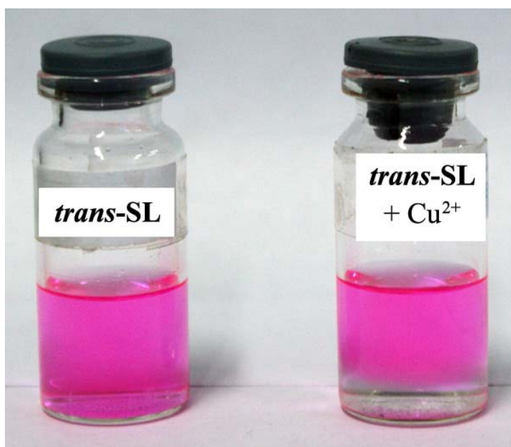
Fig. S15. Photographs of trans -SL ( 1.0 \times 10^{-5} \text{ mol dm}^{-3} in MeCN) without and with adding one drop ( 5 \times 10^{-6} \text{ dm}^{-3} ) of \text{Cu}^{2+} ( 2.0 \times 10^{-2} \text{ mol dm}^{-3} in \text{H}_2\text{O} ) immediately.
