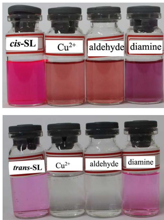
Fig. S11. Photographs of cis -SL and trans -SL (from left to right: SL; SL + 1.0 equiv. of Cu 2+ ; SL + 1.0 equiv. of 4-(diethylamino)-2-hydroxybenzaldehyde + 1.0 equiv. of Cu 2+ ; SL + 1.0 equiv. of 2,3-diaminomaleonitrile + 1.0 equiv. of Cu 2+ ).
