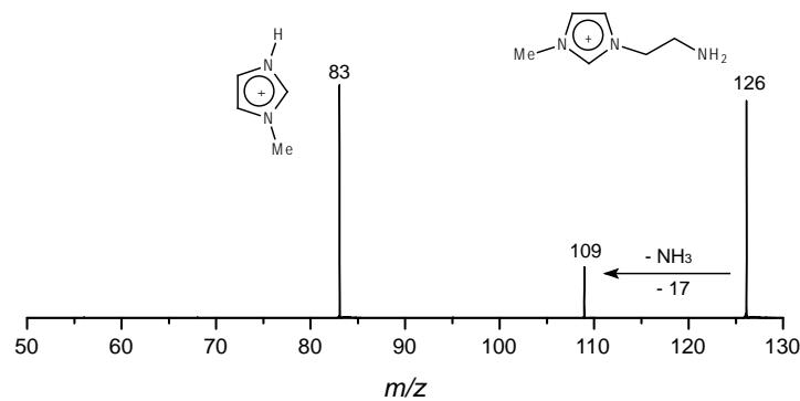
**Figure S5.** ESI(+)-MS/MS of the signal of the charge-tagged amine.
