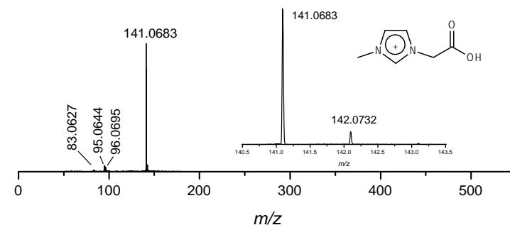
**Figure S2.** ESI(+) MS/MS from a methanolic solution of the charge-tagged carboxylic acid 1-methyl-3-carboxymethylimidazolium chloride (**MAI.Cl**). Note that the ion of  $m/z$  141 is the cation **MAI**.
