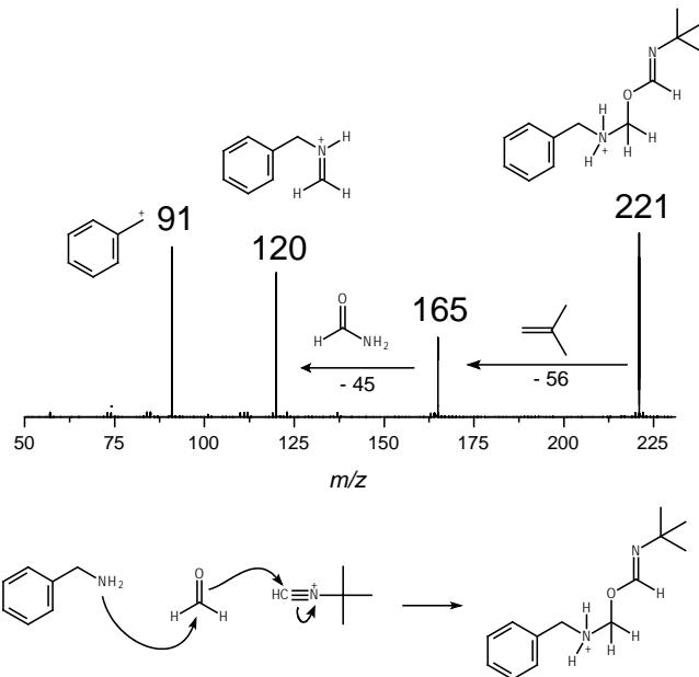
**Scheme S1.** ESI(+)-MS/MS of the by-product ion of  $m/z$  221 and (bottom) a proposal for this side reaction mechanism.
