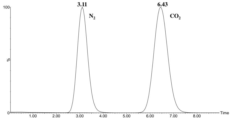
**Figure S4.** Drift time plots for the ion of  $m/z$  343. For N<sub>2</sub> as the drift gas flow: 45 mL min<sup>-1</sup> (2.19 mbar); wave velocity: 250 ms<sup>-1</sup> and wave height: 30 V. For CO<sub>2</sub> as the drift gas flow: 50 mL min<sup>-1</sup> (1.54 mbar); wave velocity: 200 ms<sup>-1</sup> and wave height: 30 V.
