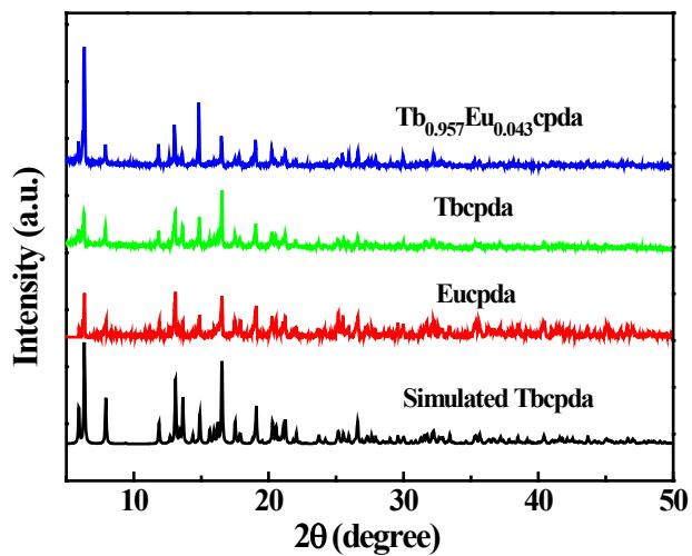
**Fig. S1** PXRD patterns of the coordination polymers **Tbcpda**, **Eucpda** and **Tb<sub>0.957</sub>Eu<sub>0.043</sub>cpda**.
