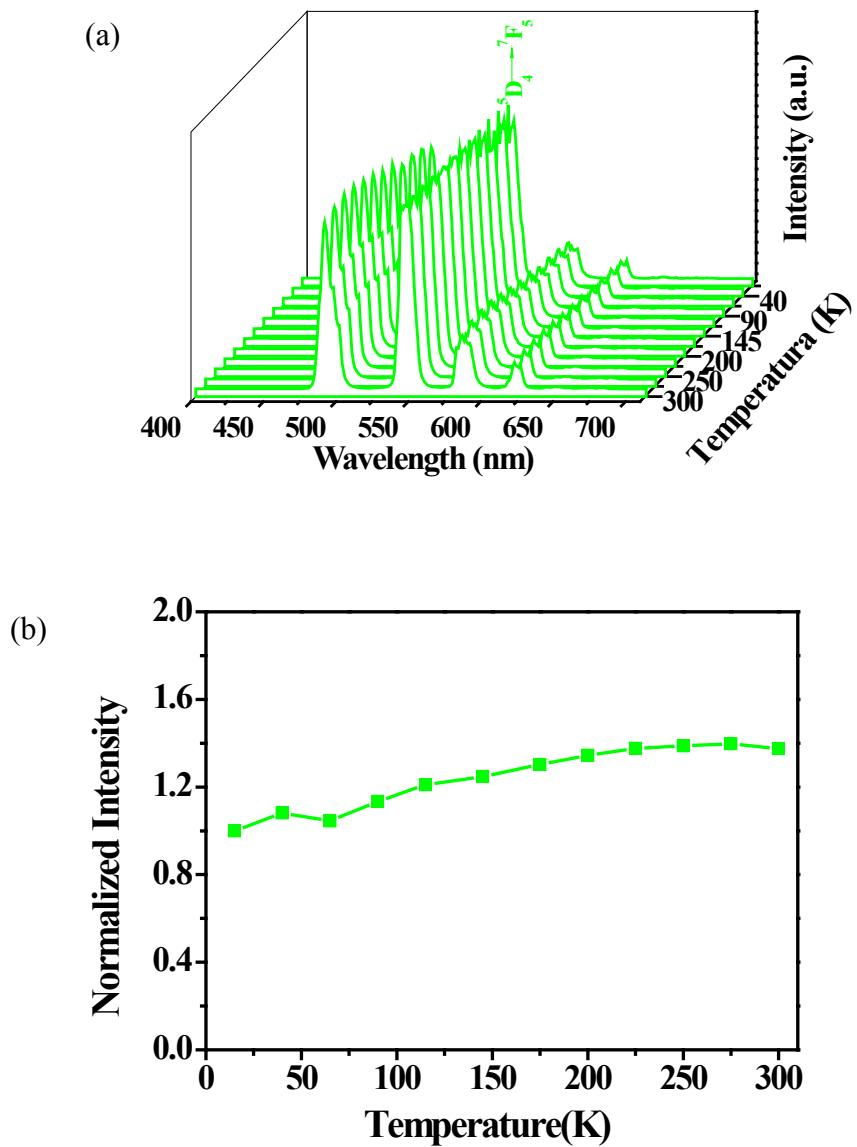
**Fig. S6** (a) Emission spectra of **Tbcpda** recorded between 15 and 300 K excited at 335 nm; (b) Temperature-dependent intensity of the  $^5D_4 \rightarrow ^7F_5$  transition of **Tbcpda**.
