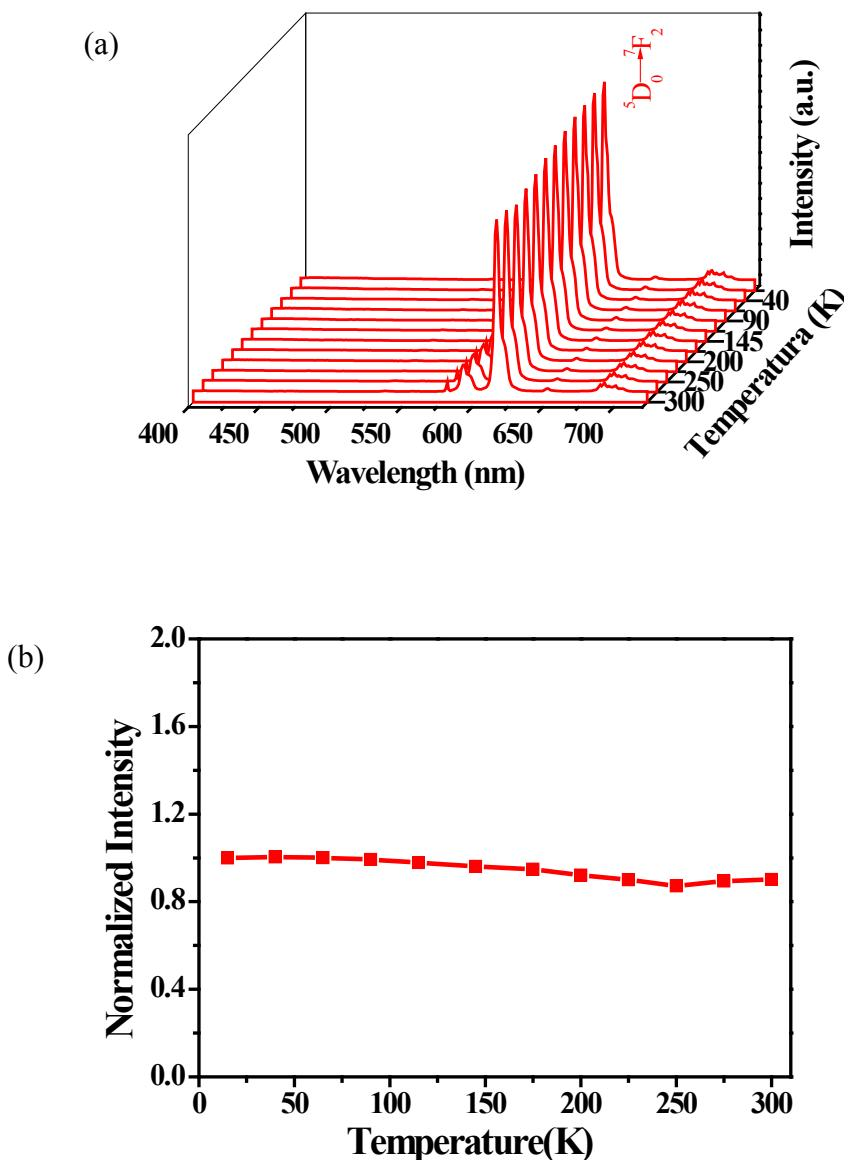
**Fig. S7** (a) Emission spectra of **EuCPDA** recorded between 15 and 300 K excited at 328 nm; (b) Temperature-dependent intensity of the  ${}^5D_0 \rightarrow {}^7F_2$  transition of **EuCPDA**.
