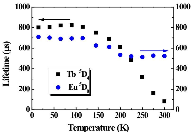
**Fig. S10** Temperature dependence of the  ${}^5\text{D}_4$  and  ${}^5\text{D}_0$  lifetime (15–300 K) for  $\text{Tb}_{0.957}\text{Eu}_{0.043}\text{cpda}$ .
