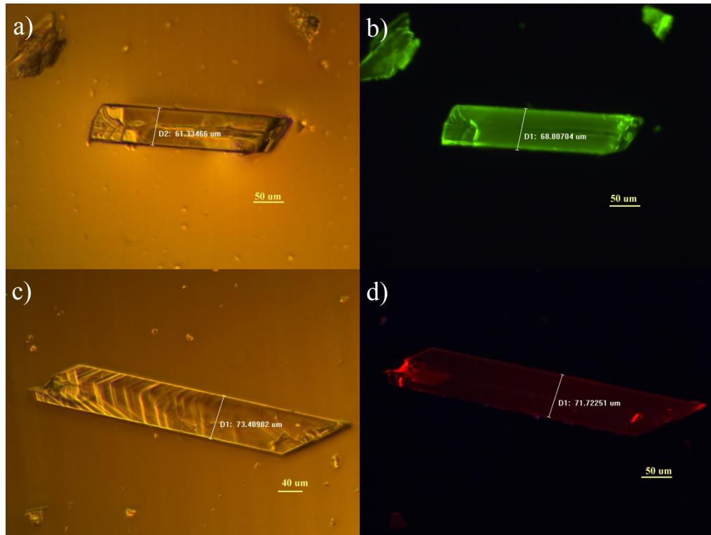
**Fig. S3** Fluorescent microscope images of **Tbcpda** illuminated with mercury lamp (a) and 365nm UV light (b) and **Tb<sub>0.957</sub>Eu<sub>0.043</sub>cpda** illuminated with mercury lamp (c) and 365nm UV light (d).
