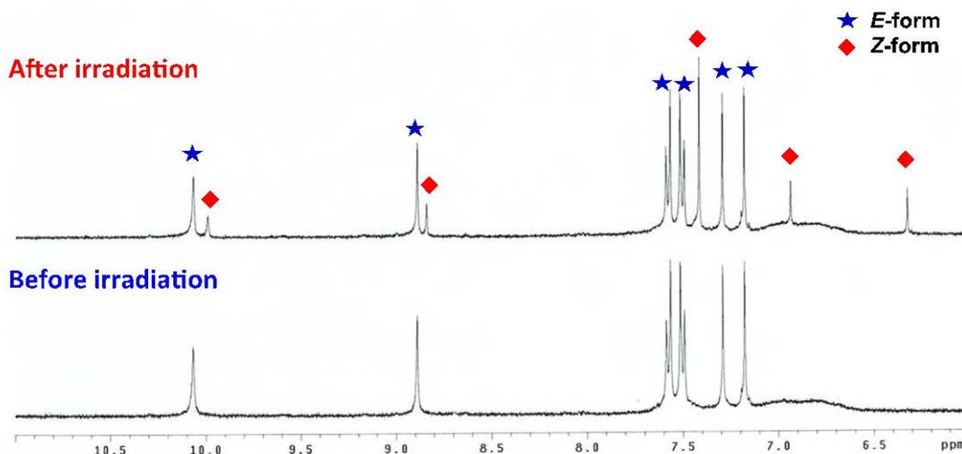
Figure S3. The NMR spectra of compound 1 before and after irradiation for 2 hr (1000 W).
