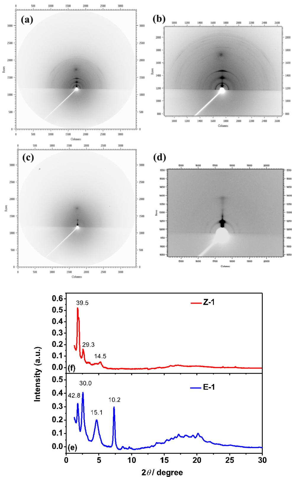
Figure S6. GIXS patterns of (a, b) *E-1* and (c, d) *Z-1* in self-assembled states. The magnification images are displayed in (b) and (d). XRD patterns of (e) *E-1* nanofibers, and (f) *Z-1* nanospheres.
