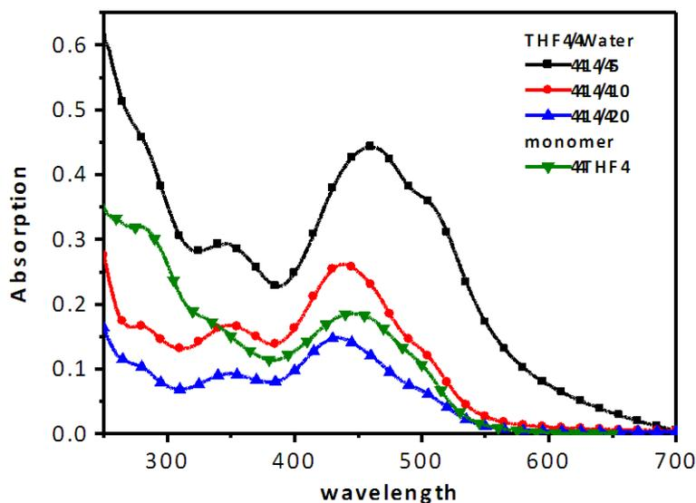
Figure S9. Absorption spectra of compound **1** in different volume ratio of THF/H<sub>2</sub>O system from 1/5 to 1/20 compared with monomer in pure THF solution (10<sup>-5</sup> M).
