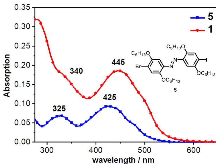
Figure S1. UV/Vis spectra of compounds 1 and 5 in THF solution ( $10^{-5}$  M).
