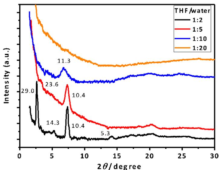
Figure S10. XRD patterns of compound **1** self-assembled in different volume ratio of THF/H<sub>2</sub>O system from 1/2 to 1/20. Two strong peaks at 29.0 Å, 10.4 Å and two weak peaks at 14.3 Å, 5.3 Å in the small-angle region are attributed to a rectangular columnar arrangement.<sup>1</sup> Along with increasing composition of water, the peaks become weak and broad, then disappear finally.
