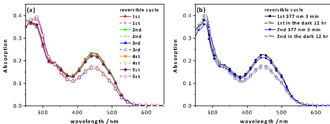
Figure S2. (a) The absorption spectra of compound E-1 after excited at 377 nm for 2 minutes (solid symbol) and then excited at 450 nm for 2 minutes (empty symbol). (b) The absorption spectra of compound E-1 after excited at 377 nm for 3 minutes (solid symbol) and stood for 12 hrs in the dark (empty symbol). A high power Xe lamp (1000 W) is used as the light source.
