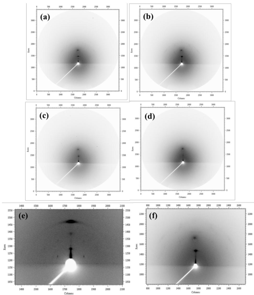
Figure S11. GIXS patterns of compound **1** self-assembled in different volume ratio of THF/H<sub>2</sub>O system from (a) 1/2, (b) 1/5, (c) 1/10 and (d) 1/20. The magnification GIXS patterns of compound **1** in (e) 1/2, (f) 1/5 THF/H<sub>2</sub>O system.
