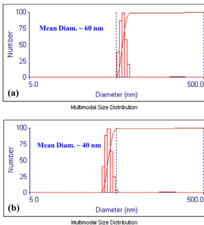
Figure S8. DLS measurement of compound **1** at THF/Water (a) 1:10 and (b) 1:20.
