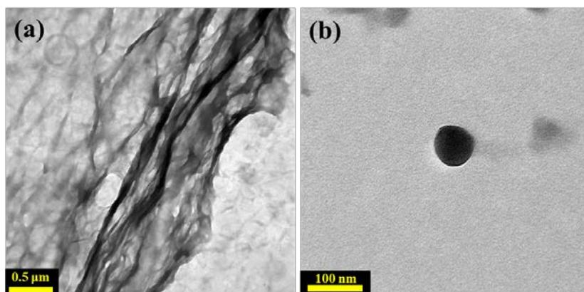
Figure S7. TEM images of compound **1** at  $10^{-4}$  M in co-solvent systems of (a) THF/Hex = 1:5 (b) TEM of THF/H<sub>2</sub>O system,  $V_{\text{THF}} / V_{\text{water}} = 1/20$
