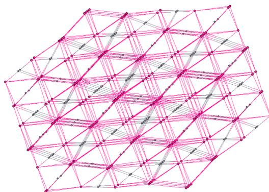
**Fig. S5.** (4, 12)-connected network of MMPF-9 (gray, 4-connected node; pink, 12-connected node).
