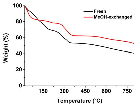
**Fig. S7.** Thermogravimetric analysis plots of MMPF-9.
