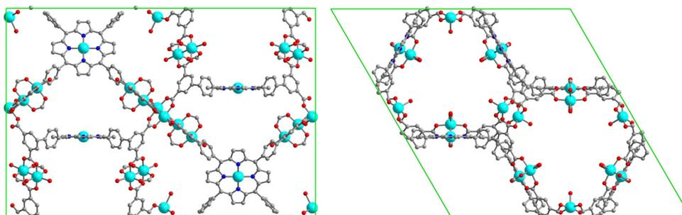
**Fig. S4.** Unit cell along *a* (left) or *b* (right) axis (copper sites are highlighted as turquoise balls).
