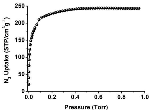
Fig. S8. N<sub>2</sub> adsorption isotherm of MMPF-9 at 77 K.
