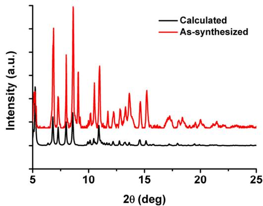
**Fig. S6.** Powder X-ray diffraction patterns of MMPF-9.
