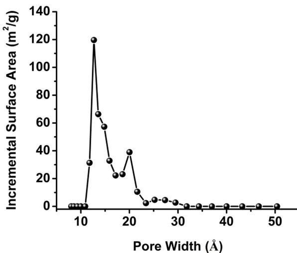
Fig. S9. Pore size distribution of MMPF-9 based on N<sub>2</sub> adsorption isotherm at 77 K (DFT model).
