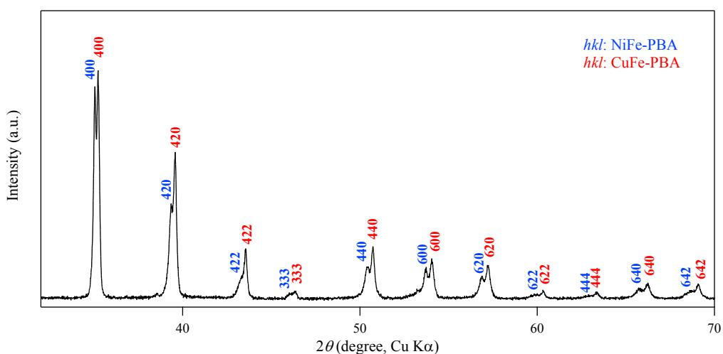
Fig. S2. Powder X-ray diffraction patterns for CuFe-PBA@NiFe-PBA.
