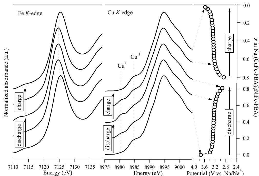
Fig. S3. *Ex situ* XANES spectra for Fe and Cu K-edges on discharge/charge of (a) CuFe-PBA and (b) CuFe-PBA@NiFe-PBA.
