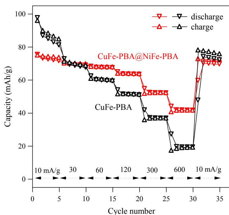
Fig. S5. Cycle stability of CuFe-PBA and CuFe-PBA@NiFe-PBA during the high charge/discharge rate experiment.
