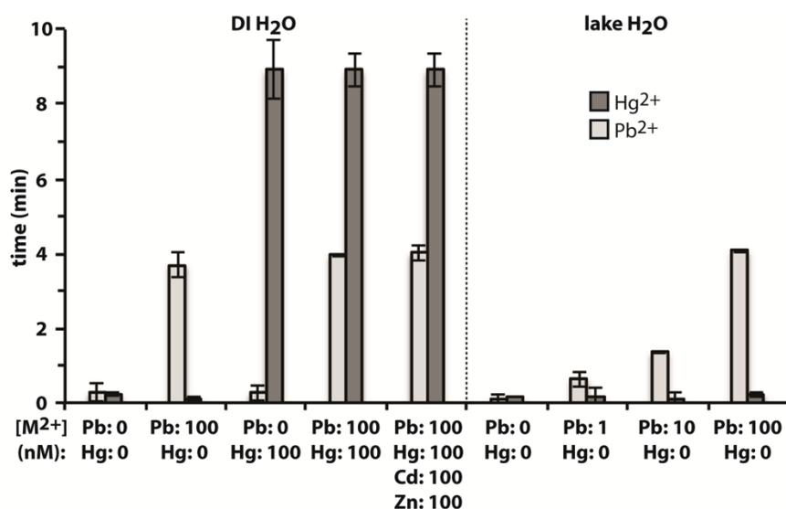
**Figure S6.** Select assay results using the four-channel device shown in Fig. 1. The values are the average of three measurements and the error bars reflect the standard deviations of these averages.
