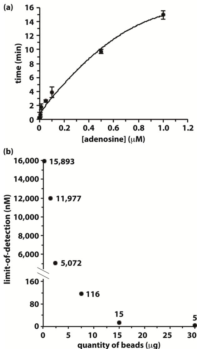
**Figure S2.** Detection of adenosine as a model target to show quantitative detection of an analyte using the aptamer-based assay. (a) Calibration curve showing the relationship between the measured time and the concentration of adenosine. (b) Tuning the sensitivity of the adenosine assay by varying the quantity of the adenosine aptamer (immobilized on microbeads) in layer 5 of the device for performing assays of a single analyte (Fig. S1).
