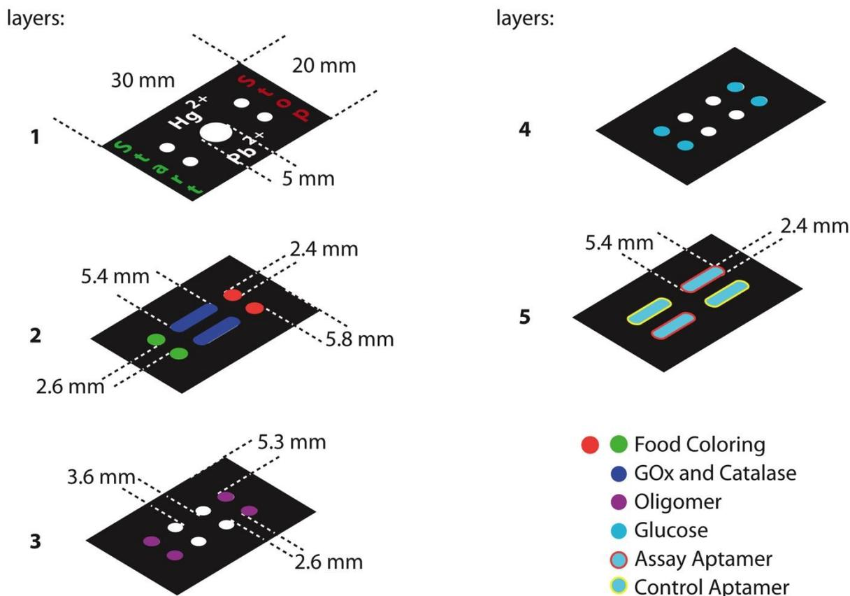
**Figure S5.** Expanded view of the device shown in Figure 1. The device is 20 mm wide  $\times$  30 mm long  $\times$  1.8 mm thick.
