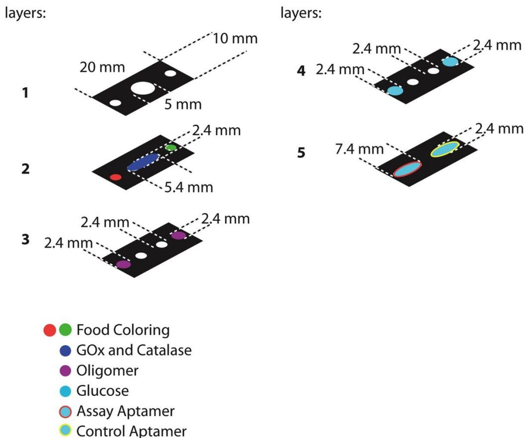
**Figure S1.** Expanded view of the two channel device. The device is 10 mm wide  $\times$  20 mm long  $\times$  1.8 mm thick.
