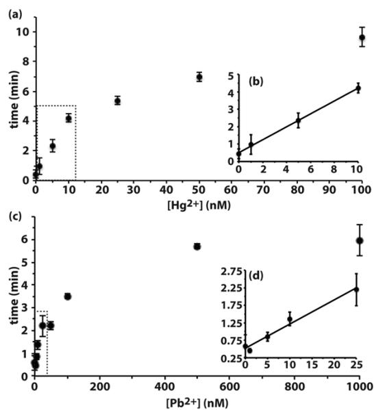
**Fig. S4** Calibration curves for (a) Hg<sup>2+</sup> and (c) Pb<sup>2+</sup> using two-channel paper-based devices. The calibration curves were obtained at 20 °C and 37% relative humidity. The data points are the average of four measurements and the error bars reflect the standard deviations of these averages. The insets (b) and (d) show the linear regions that are defined by the dotted rectangles. These linear regions were used to calculate the limits-of-detection values for the assays.
