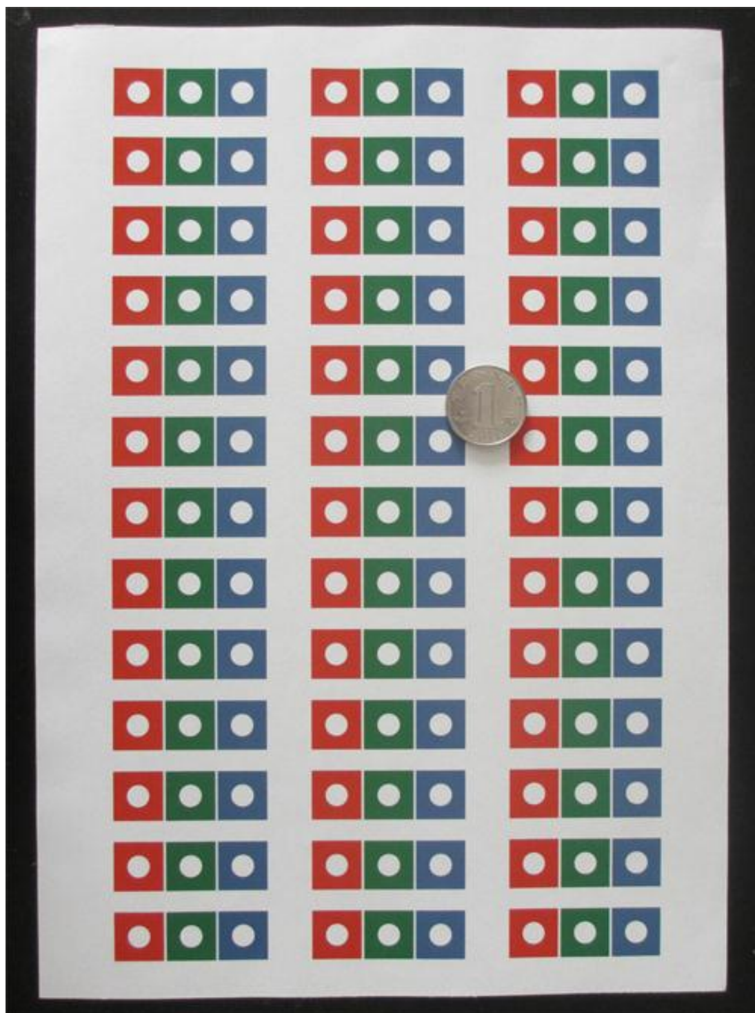
Figure S1. Wax-printed 3D- \mu -OBFCADs on a paper sheet (A4) before baking.
