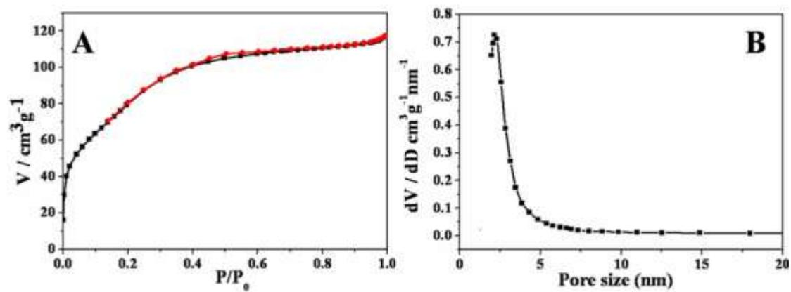
**Fig. S3.**  $\text{N}_2$  sorption isotherm curves (A) and pore size distribution plots (B) of the core-shell structured MO@MCM-41 composites prepared by using surfactant CTAB as a template.
