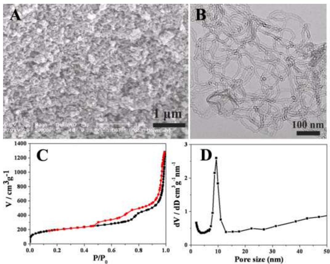
**Fig. S2.** SEM (A) and TEM images (B), the N<sub>2</sub> sorption isotherm curves (C) and pore size distribution plots (D) of the mesoporous silica nanotubes, prepared in 1.3 mol/L of boric acid medium by using Pluronic P123 as a template without the addition of magnetic oxides.
