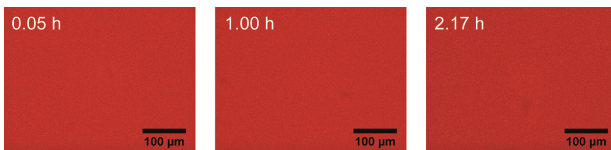
Figure S6. Fluorescence micrographs of BSA doped with 2 mol% Texas Red-conjugated BSA adsorbed at the air/buffer interface at various time points. The interfacial film was subjected to sinusoidal oscillations ( T 33 s; \Delta A 15%). The BSA concentration was: 7.5 \cdot 10^{-7} \text{ mol L}^{-1} .
