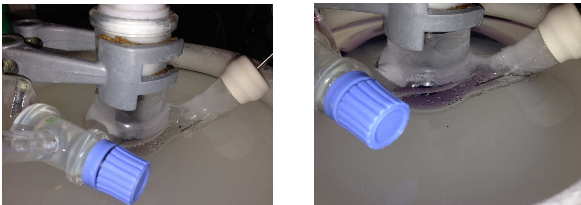
Figure 9. 3 mM Solution of [\text{Cu}(\text{I})\text{L}_{\text{py}1}(\text{CH}_3\text{CN})_2]\text{PF}_6 in anhydrous acetone at 180 K at the beginning of the oxygenation (left) and after 5 minutes of oxygenation (right); the color of the solution changes from pale yellow to deep purple.
