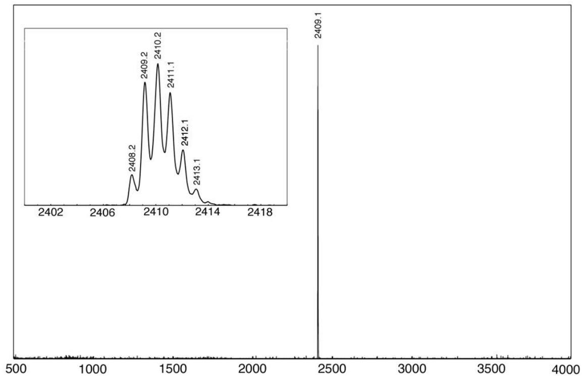
**Fig. S13.** LDI-TOF mass spectrum of **DBA-DA24.25**.
