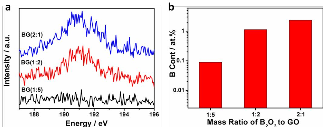
Fig. S4 (a) B1s XPS spectra of BG obtained at different mass ratios of  $\text{B}_2\text{O}_3$  to GO, (b) the B content vs the mass
