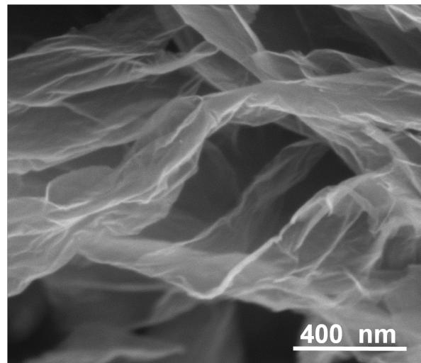
**Fig. S1** SEM image of as-prepared graphene.
