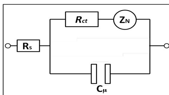
**Fig. S7** The equivalent circuit of the cell.
