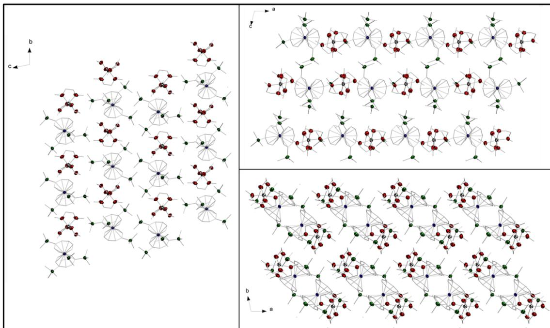
**Figure S1.** Packing arrangement of **1** looking down the *a* (left) *b* (top right) and *c* (bottom right) axis. H atoms are omitted for clarity. Color code: Si = green, Er = blue, Li = yellow, O = red, C = grey.
