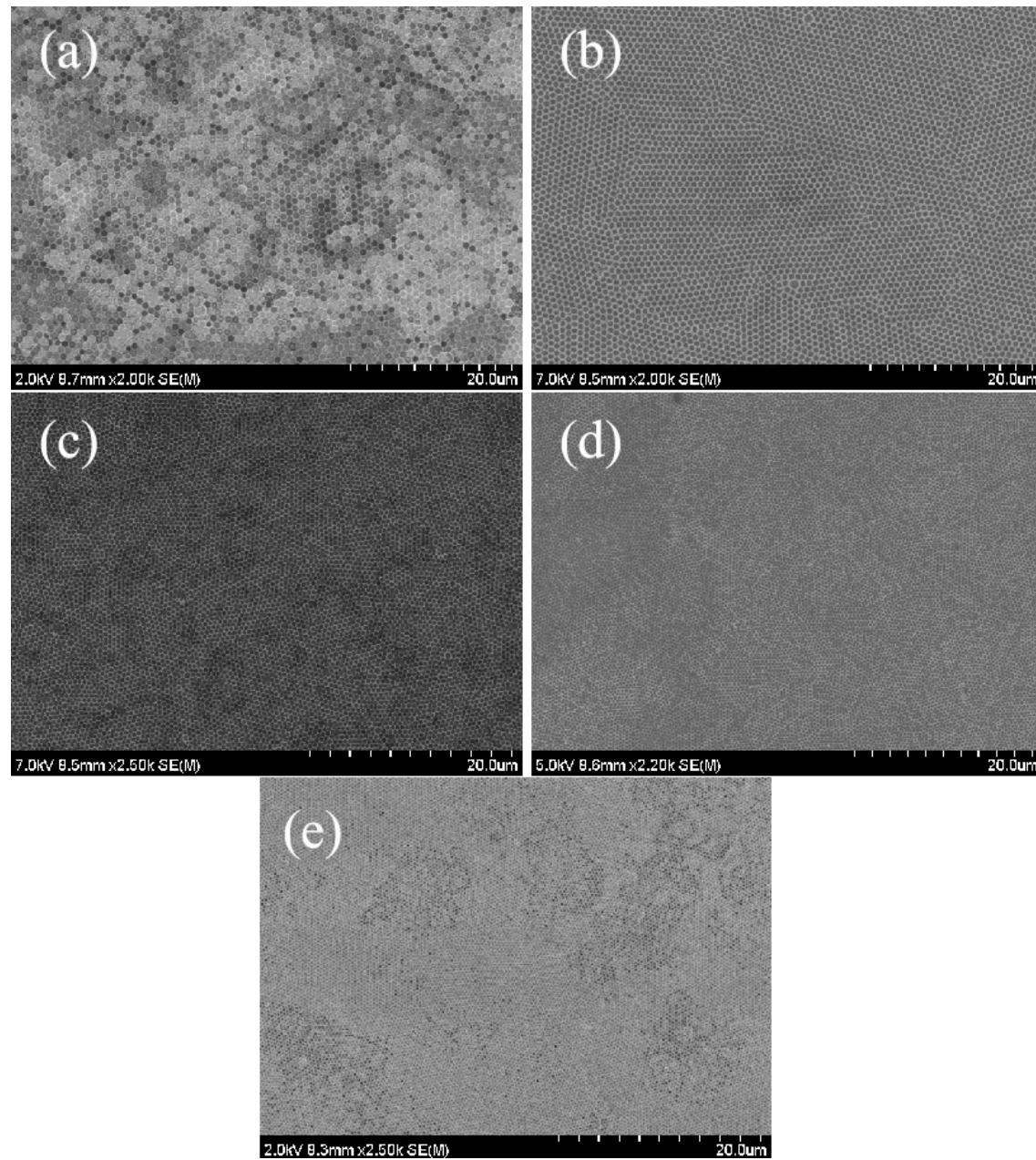
**Figure S3** SEM images of  $\text{WO}_3$  IO films templated by PS spheres of 920 nm (a); 880 nm (b); 530 nm (c); 480 nm (d) and 410 nm (e), showing crack-free samples.
