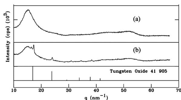
**Figure S6** XRD patterns of WO<sub>3</sub>880 IO sample heated at 150 °C (a) and 400 °C (b) showing amorphous WO<sub>3</sub> at 150 °C, and crystalline WO<sub>3</sub> (PDF-41-0905) at 400 °C.
