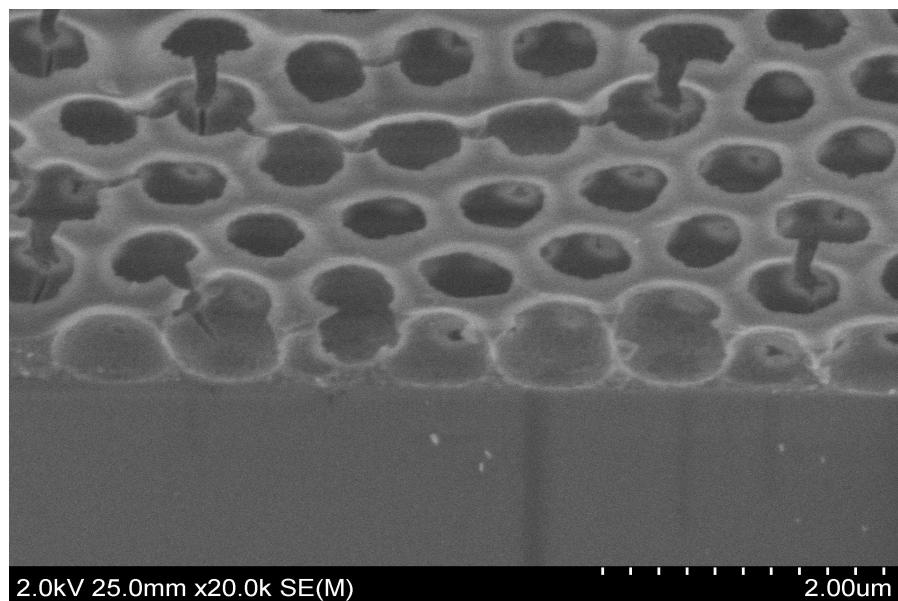
**Figure S2.** Cross-sectional scanning electron microscope image of a  $\text{WO}_3$  IO film templated by PS spheres of 880 nm diameter. (Sample tilted at 47 °)
