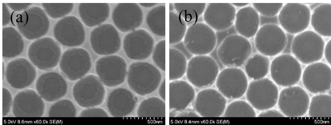
**Figure S1** SEM images of  $\text{WO}_3$  IO films on ITO substrates templated by 480 nm PS spheres: 8.0 ml (a) and 7.0 ml (b) of  $\text{WO}_3$  solution used for the PS opals formed with 0.3 ml PS solution (0.5 %w/v).
