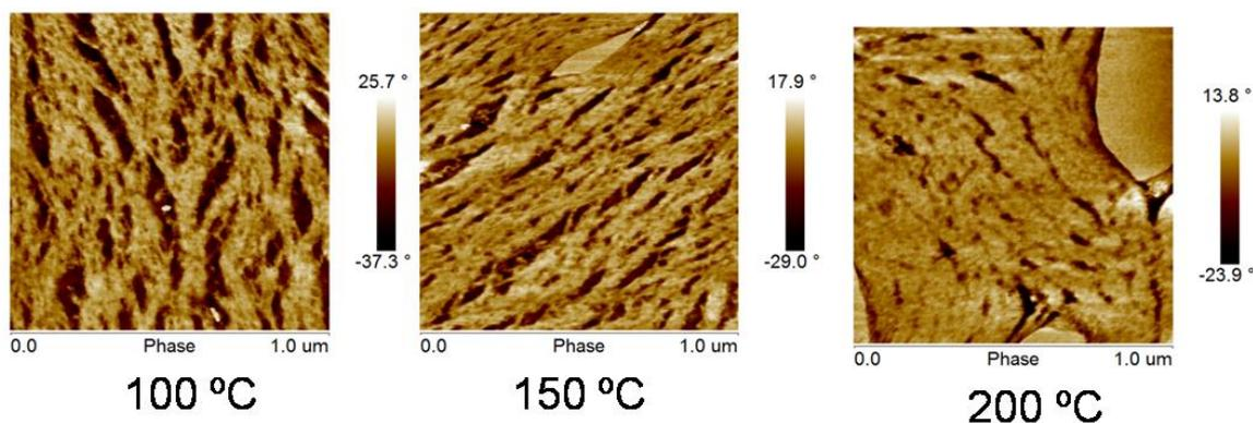
**Fig. S3** AFM phase and topography images of PBIBDF-BT at different annealing temperature.
