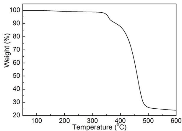
**Fig. S5** TGA plot of PBIBDF-BT.
