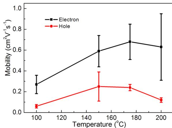
**Fig. S1** Effects of the annealing temperature on electron and hole mobilities of PBIBDF-BT.
