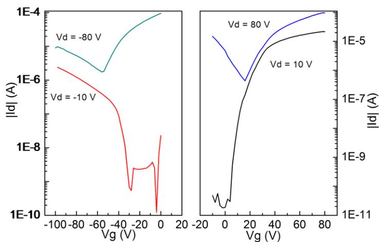
**Fig. S2** Typical transfer characteristic of annealing OTFTs devices based on PBTBDF-BT after three months' air exposure.
