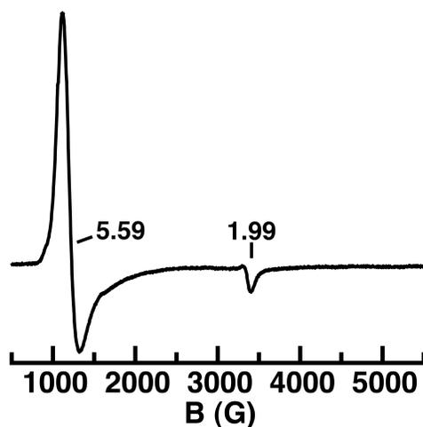
**Fig. S2** Perpendicular-mode X-band EPR spectrum of 9.8 mM Fe<sup>III</sup>MST(NH<sub>3</sub>) collected as a frozen glass in 1:1 DCM:THF at 77K.
