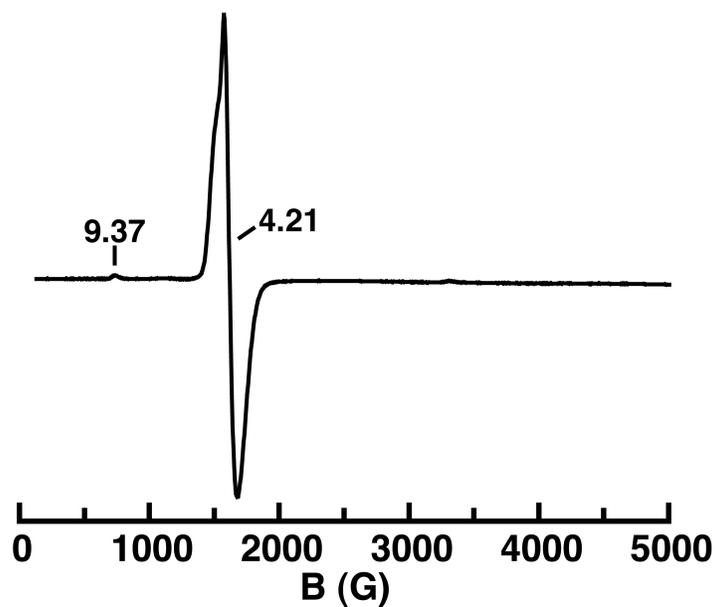
**Fig. S9** Perpendicular-mode X-band EPR spectrum of 9.8 mM  $[\text{Fe}^{\text{III}}\text{MST}(\text{NH}_3)]$  after treatment with TBD, collected as a frozen glass in 1:1 DCM:THF at 77K.
