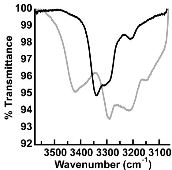
**Fig. S10** Solution FTIR spectra of 9.8 mM [Fe<sup>III</sup>MST(NH<sub>3</sub>)]<sup>-</sup> before (black line) and after (gray line) treatment with TBD. Spectra collected in 1:1 DCM:THF at 298 K. Note:  $\nu(\text{NH})$  peaks at 3289, 3213, and 3153 cm<sup>-1</sup> for the gray line are from TBD.
