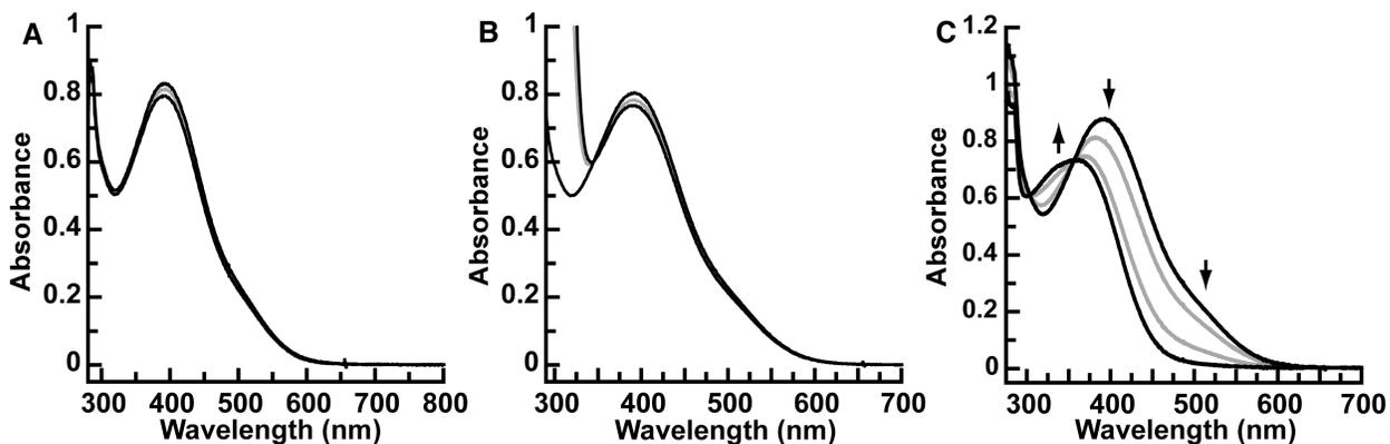
**Fig. S8** Electronic absorption spectra of  $[\text{Fe}^{\text{III}}\text{MST}(\text{NH}_3)]$  treated with an excess of pyrrolidine (**A**) 2-phenyl-1,1,3,3-tetramethylguanidine (**B**) or 1,8-diazabicyclo[5.4.0]undec-7-ene (**C**). Spectra were collected in DMSO at 298 K.
