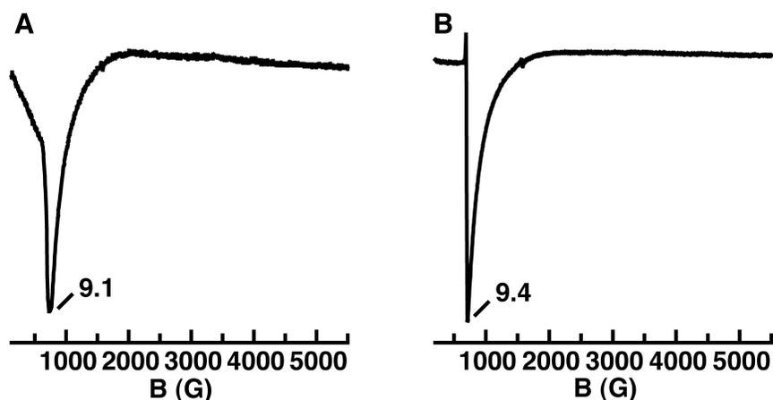
**Fig. S1** Parallel-mode X-band EPR spectra of Na[Fe<sup>II</sup>MST] (A) and Na[Fe<sup>II</sup>MST(NH<sub>3</sub>)] (B), each collected as a frozen glass in 1:1 DMA:THF at 10 K.
