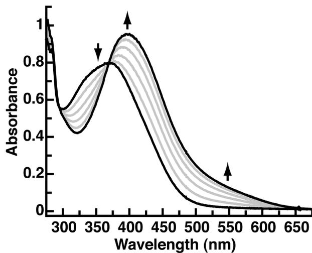
**Fig. S11** Electronic absorption spectrum of [Fe<sup>III</sup>MST(NH<sub>2</sub>)]<sup>-</sup> in THF treated with HNEt<sub>3</sub>BF<sub>4</sub> at 298 K.
