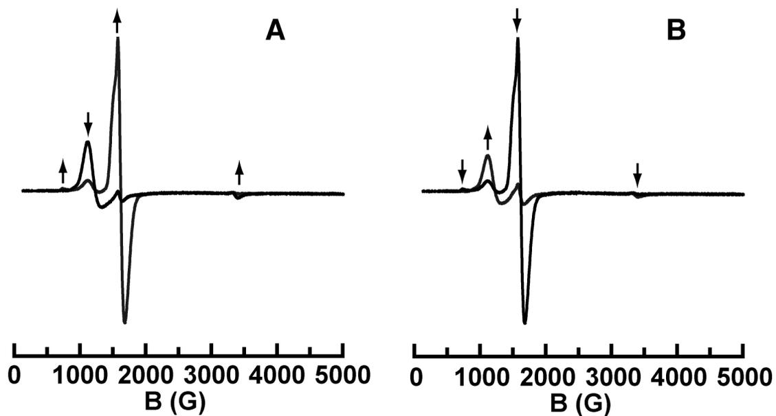
**Fig. S12** Perpendicular-mode X-band EPR spectra of 9.8 mM [Fe<sup>III</sup>MST(NH<sub>3</sub>)] before and after addition of TBD (**A**) and regeneration of the [Fe<sup>III</sup>MST(NH<sub>3</sub>)] signal after the addition of HNEt<sub>3</sub>BF<sub>4</sub> (**B**). The sample was collected as a frozen glass in 1:1 DCM:THF at 77 K.
