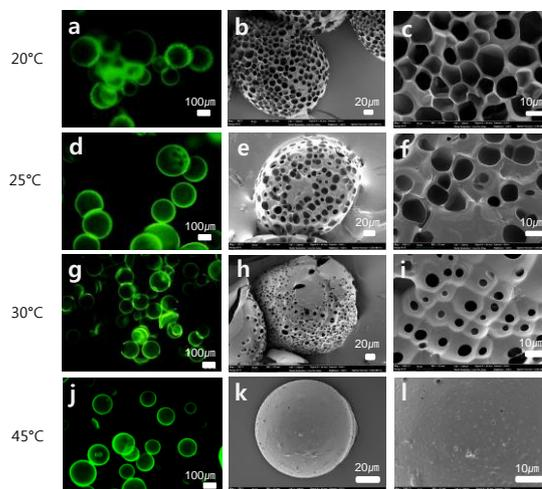
**Fig. S1.** Morphological variations between the ELP microcapsules prepared at different crosslinking temperatures. Microcapsules were prepared at (a-c) 20°C, (d-f) 25°C, (g-i) 30°C and (j-l) 45°C. (a, d, g, i) Confocal images, (b, e, h, k) FE-SEM images and (c, f, i, l) enlarged FE-SEM images of microcapsules.
