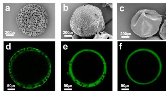
**Fig. S2.** Morphological variations of the ELP microcapsules prepared at different maturation time. FE-SEM images of microcapsules prepared after the maturation for (a) 15 min, (b) 30 min and (c) 60 min. (d-f) Confocal images of a-c. Microcapsules were prepared at 45°C.
