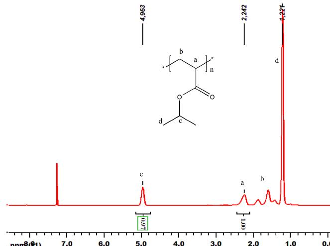
**Fig. S9** <sup>1</sup>H NMR spectrum (CDCl<sub>3</sub>, 400 MHz) of poly (isopropyl acrylate) obtained via one pot strategy.
