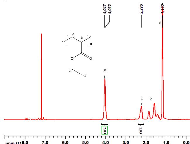
**Fig. S6** <sup>1</sup>H NMR spectrum ( $\text{CDCl}_3$ , 400 MHz) of poly(ethyl acrylate) obtained via one pot strategy.
