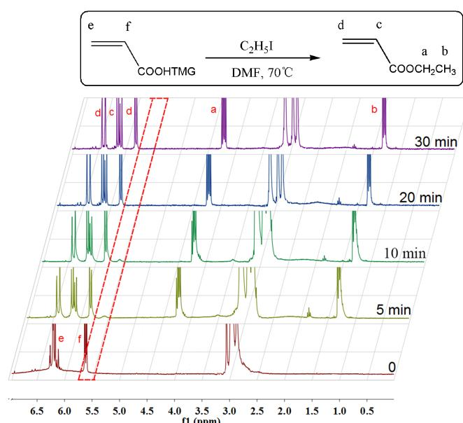
**Fig. S1**  $^1\text{H}$  NMR spectra of the TMG promoted esterification reaction of acrylic acid with ethyl iodide at 70°C at different reaction time. The signals between 2.5 and 3.5 ppm are assigned to methyl protons of DMF and TMG salt.
