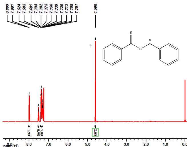
**Fig. S5** <sup>1</sup>H NMR spectrum ( $\text{CDCl}_3$ , 400 MHz) of benzyl dithiobenzoate.
