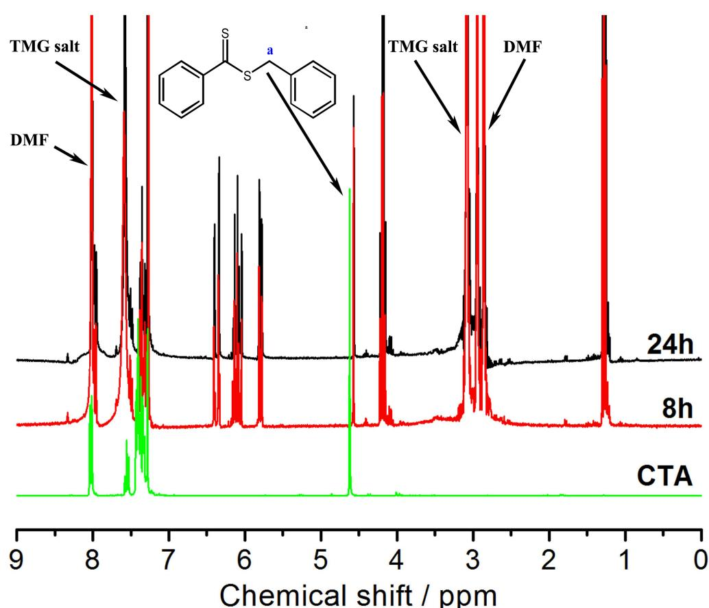
Fig. S13 The  $^1\text{H}$  NMR spectrum of polymerization mixture (acrylic acid, TMG, ethyl iodide, and CTA in DMF ) after reaction for 8h or 24h at 70°C
