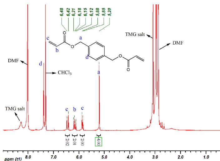
**Fig. S3** <sup>1</sup>H NMR spectrum (CDCl<sub>3</sub>, 400 MHz) of the TMG promoted esterification reaction of acrylic acid with 1,4-bis (bromomethyl) benzene at 70°C in DMF. The sample was withdrawn after reaction for **5 min** and dissolved in CDCl<sub>3</sub> for <sup>1</sup>H NMR analyse. The yield is 100% calculated according the spectrum.
