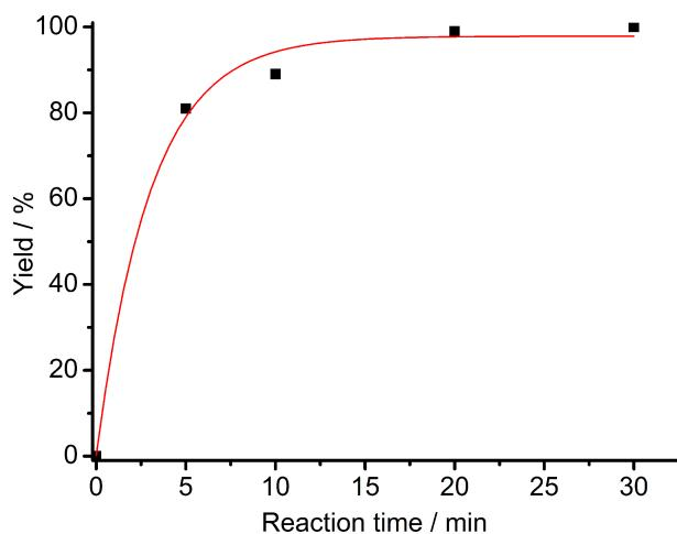
**Fig. S2** Plot of product yield versus reaction time for the reaction of acrylic acid with ethyl iodide in DMF using TMG as promoter at 70°C
