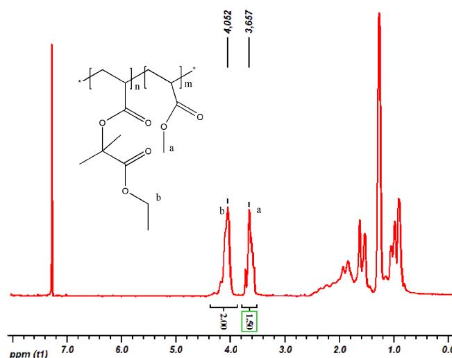
**Fig. S11** <sup>1</sup>H NMR spectrum (CDCl<sub>3</sub>, 400 MHz) of poly (1-ethoxy-2-methyl-1-oxopropan-2-yl acrylate-block-methyl acrylate) after methylation of poly (1-ethoxy-2-methyl-1-oxopropan-2-yl acrylate) with methyl iodide obtained via one pot strategy.
