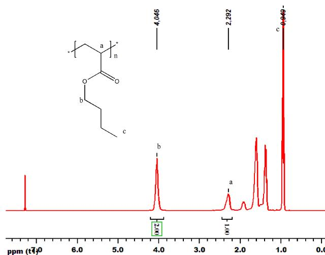
**Fig. S10** <sup>1</sup>H NMR spectrum (CDCl<sub>3</sub>, 400 MHz) of poly (n-butyl acrylate) obtained via one pot strategy.
