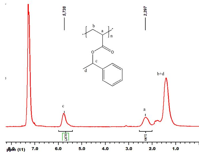
**Fig. S8** <sup>1</sup>H NMR spectrum (CDCl<sub>3</sub>, 400 MHz) of poly (1-phenylethyl acrylate) obtained via one pot strategy.
