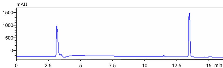
**Figure S3.** HPLC spectrum of pentafluorophenol activated platinum(IV) complex at absorbance of 214 nm.
