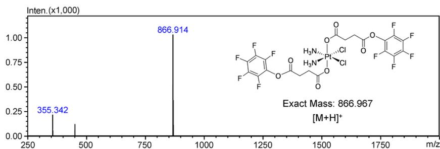
**Figure S5.** Mass spectrum (IT-TOF) of pentafluorophenol activated platinum(IV) complex.
