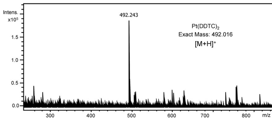
**Figure S15.** Mass spectrum (ESI) of Pt(DDTC)<sub>2</sub> formed from the adduction of DDTC with the reduced prodrug.
