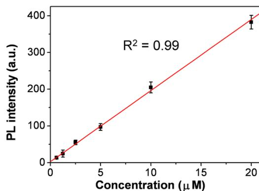
**Figure S20.** Plot of PL intensity at 605 nm versus concentrations of PyTPE-Pt-D5 with the incubation of ascorbic acid (1 mM) in DMSO/PBS (v/v = 1/199). Data represent mean values  $\pm$  standard deviation, n = 3.
