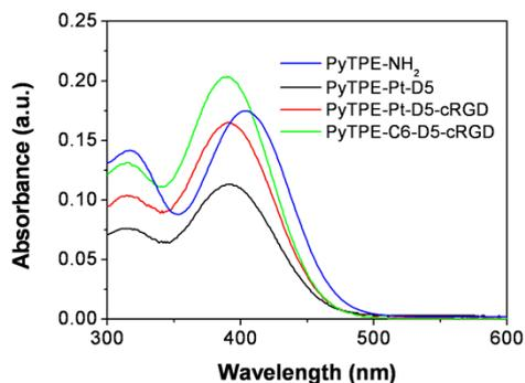
**Figure S17.** (A) UV-vis absorption spectra of PyTPE-NH<sub>2</sub> (in THF) and PyTPE-Pt-D5, PyTPE-Pt-D5-cRGD and PyTPE-C6-D5-cRGD (in DMSO/PBS (v/v = 1/199)).
