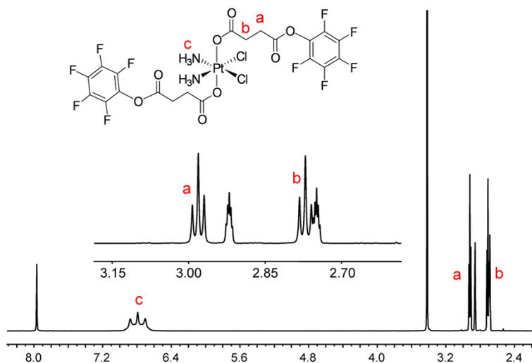
**Figure S4.**  $^1\text{H}$  NMR spectrum of pentafluorophenol activated platinum(IV) complex in  $\text{DMF-}d_7$ . An expanded view is inserted in the figure.
