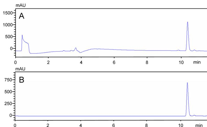
**Figure S9.** HPLC spectra of PyTPE-Pt-D5 monitored with absorbance at 214 nm (A) and 365 nm (B).
