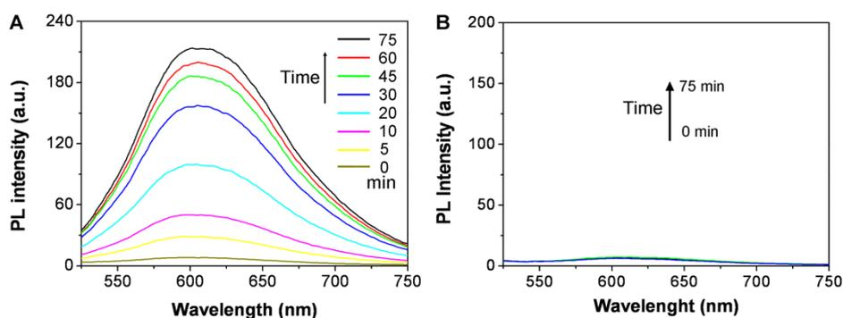
**Figure S18.** Time-dependent fluorescence spectra of PyTPE-Pt-D5 (A) and PyTPE-C6-D5-cRGD (B) (10  $\mu$ M) upon treatment with ascorbic acid (1 mM) in DMSO/PBS (v/v = 1/199).
