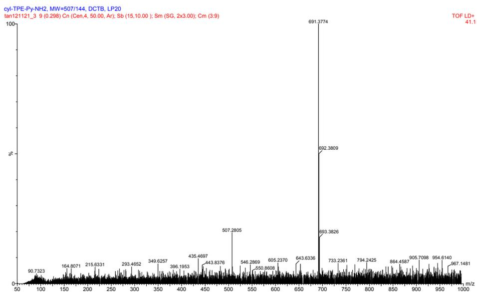
Figure S2. High resolution mass spectrum (MALDI-TOF) of PyTPE-NH<sub>2</sub>.
