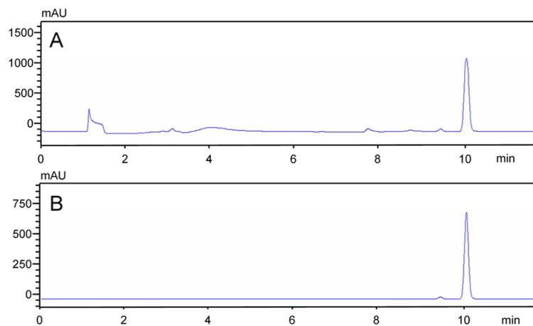
**Figure S6.** HPLC spectra of PyTPE-Pt-D5-cRGD monitored with absorbance at 214 nm (A) and 365 nm (B).
