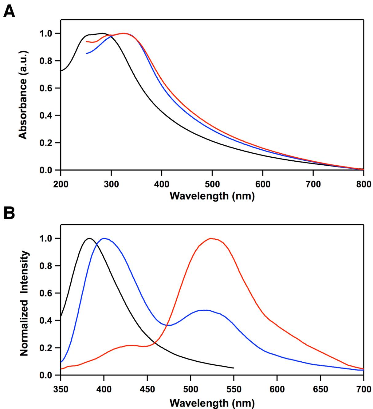
**Figure S4.** (A) Electronic absorption spectra and (B) fluorescence spectra of PP-CMP@*mmm* (black), PP-CMP@*omp* (blue) and PP-CMP@*omom* (red) dispersed in THF at 25 °C.
