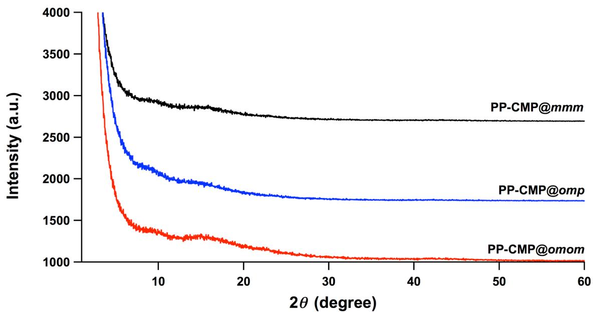
**Figure S3.** Powder X-ray diffraction profiles of PP-CMP@*mmm*, PP-CMP@*omp* and PP-CMP@*omom*. These CMPs exhibited very weak halo peaks, indicating their amorphous structure.
