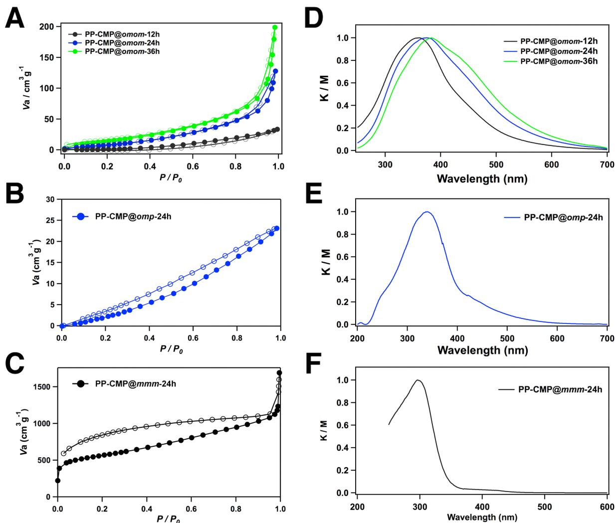
**Figure S5.** Nitrogen sorption isotherm profiles of (A) PP-CMP@*omom*-12h, PP-CMP@*omom*-24h and PP-CMP@*omom*-36h, (B) PP-CMP@*omp*-24h and (C) PP-CMP@*mmm*-24h. Electronic absorption spectra of (D) PP-CMP@*omom*-12h, PP-CMP@*omom*-24h and PP-CMP@*omom*-36h, (E) PP-CMP@*omp*-24h and (F) PP-CMP@*mmm*-24h.
