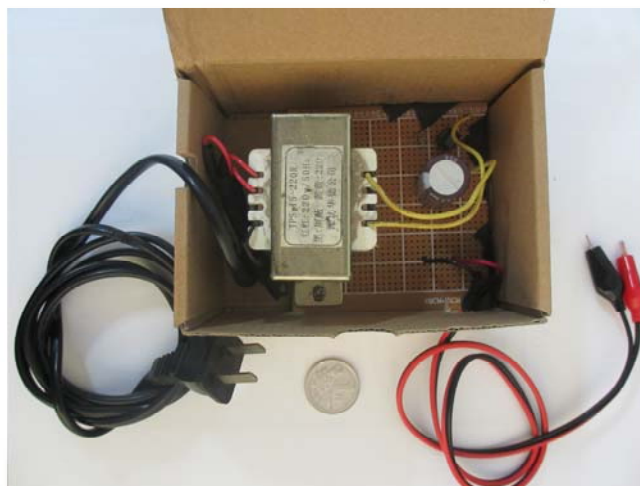
Scheme S1. Detail circuit diagram and picture of this rectifier.
